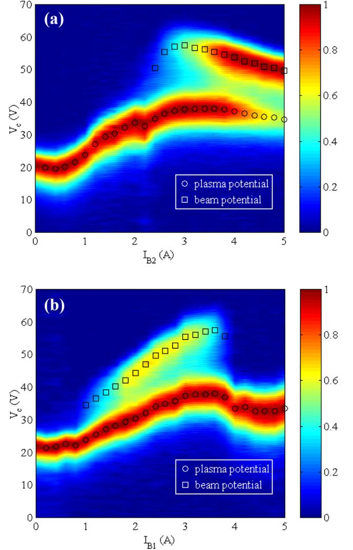
Fig. 6 (Color online) Contour plots of the normalized IEDFs (a) as a function of  $I_{B2}$  for  $I_{B1} = 3$  A, and (b) as a function of  $I_{B1}$  for  $I_{B2} = 3$  A, namely, the data are measured under the magnetic-field configurations presented in Figs. 5(a) and 5(b). The open squares and the open circles in Figs. 6(a) and 6(b) indicate the local plasma potential  $\phi_p$  and the ion beam potential  $\phi_{beam}$ , respectively.
