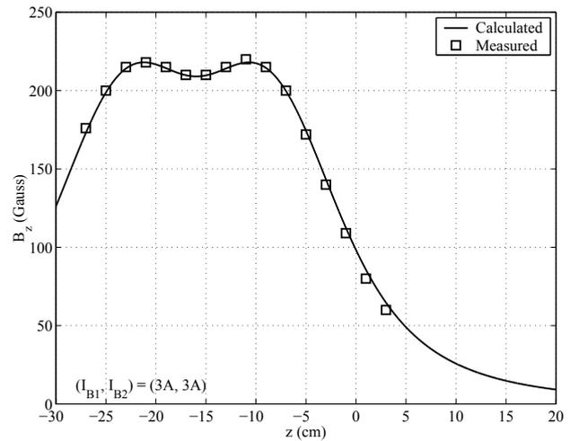
Fig. 3 The measured (open squares) and calculated (solid line) axial profiles of the axial component  $B_z$  of the magnetic-field strength for  $(I_{B1}, I_{B2}) = (3 \text{ A}, 3 \text{ A})$ .
