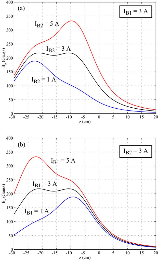
Fig. 5 (Color online) Axial profiles of the calculated magnetic-field strength  $B_z$  (a) as a function of  $I_{B2}$  for  $I_{B1} = 3$  A, and (b) as a function of  $I_{B1}$  for  $I_{B2} = 3$  A.
