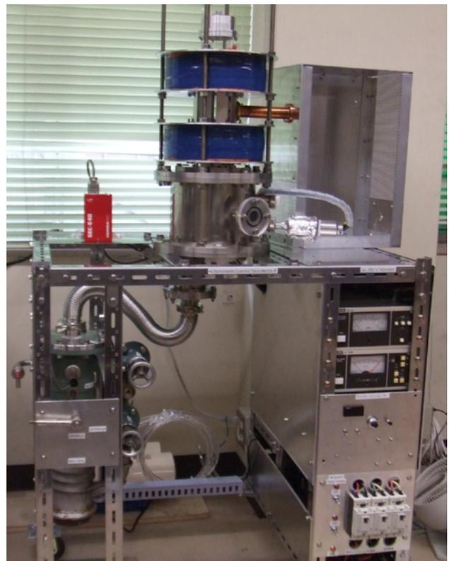
Fig. 1 (Color online) (a) Photograph of the presently-manufactured magnetically-expanding plasma device using electromagnets with 6.5-cm-diameter source tube.
