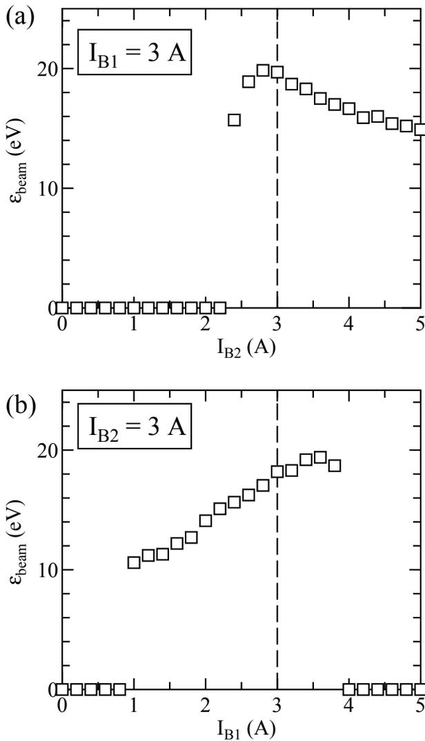
Fig. 7 Ion beam energy  $\varepsilon_{beam}$  (a) as a function of the exhaust-coil current  $I_{B2}$  for  $I_{B1} = 3$  A, and (b) as a function of the upstream-coil current  $I_{B1}$  for  $I_{B2} = 3$  A.
