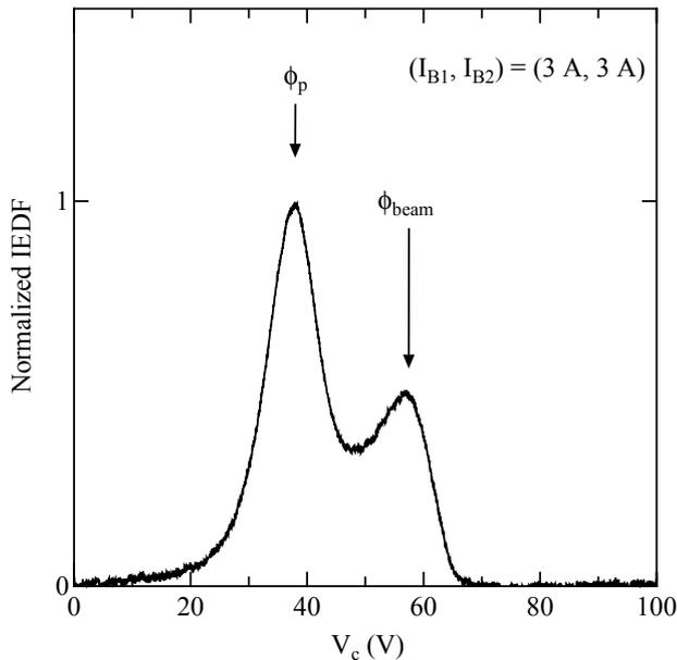
Fig. 4 The measured IEDF at  $z = 3$  cm downstream of the source exit for  $(I_{B1}, I_{B2}) = (3 \text{ A}, 3 \text{ A})$ .
