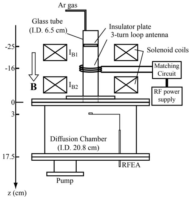
Fig. 2 Schematic diagram of the magnetically-expanding plasma device using electromagnets with 6.5-cm-diameter source tube.
