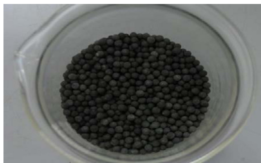
Fig.1 Appearance of Pt/ASDBC catalysts
