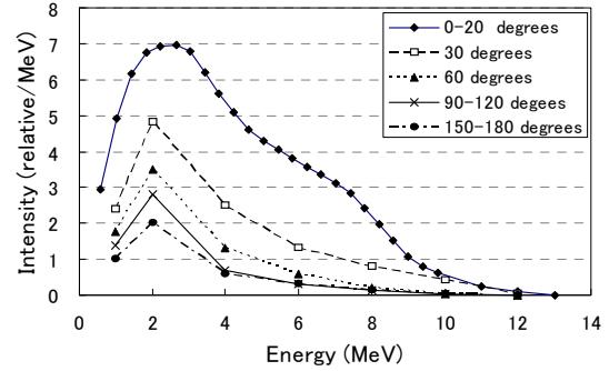
Fig. 2 Neutron energy spectra.
