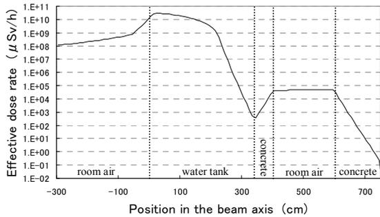
Fig. 6 Effective dose rate in the axis direction. The origin of x-axis is located at the entrance of the beam dump cone.
