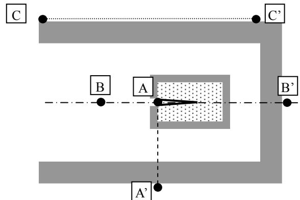
Fig. 4 Calculation positions. (A-A') : Radial direction, (B-B') : Axis direction, (C-C') : Outside of vault.
