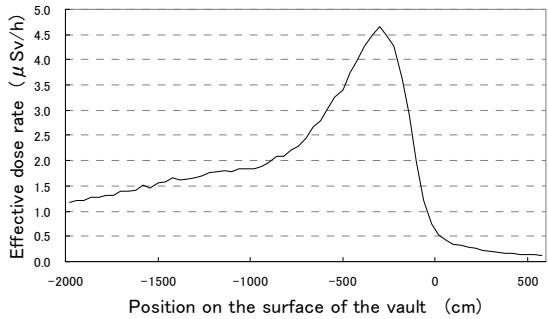
Fig. 7 Effective dose rate outside the vault. The origin of x-axis is located at the entrance of the beam dump cone.
