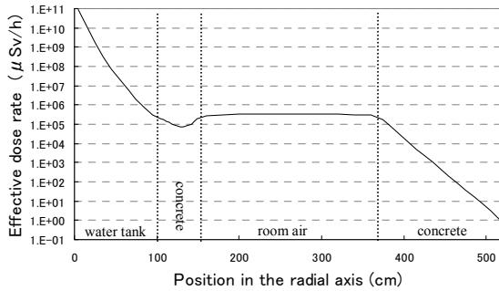
Fig. 5 Effective dose rate in the radial direction.
