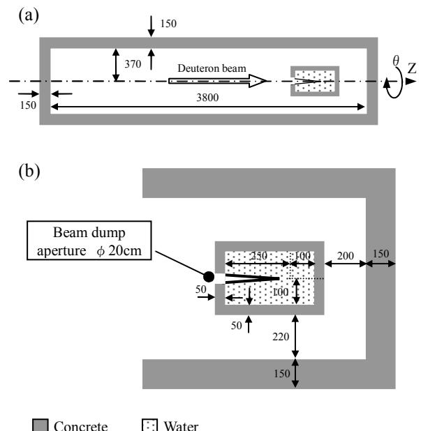
Fig. 1 Calculation model (Unit: cm)
