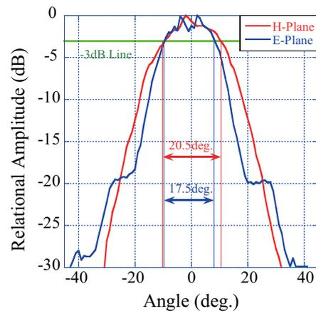
Fig. 4 Radiation Pattern of the MIR antenna element.
