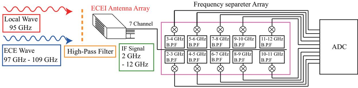
Fig. 7 Receiving Circuit of the ECEI system.
