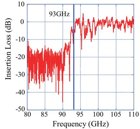
Fig. 9 Cutoff response of dichroic filter.
