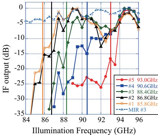
Fig. 8 Cutoff response of the test antenna.
