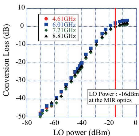
Fig. 6 Conversion losses of the MIR antenna element.
