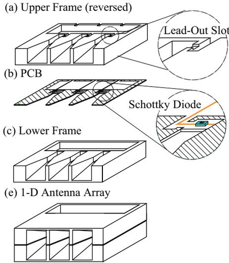
Fig. 2 Schematic view of the 1-D horn antenna array assembly. (a) underside view of upper structure, (b) PCB, (c) lower structure, (d) completed form
