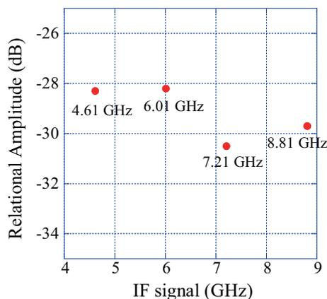
Fig. 5 Frequency Responses of the MIR antenna element.
