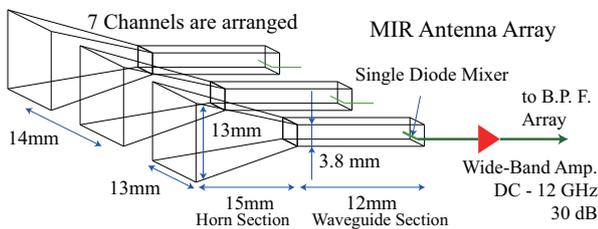
Fig. 3 Schematic view of the 1-D horn antenna array.
