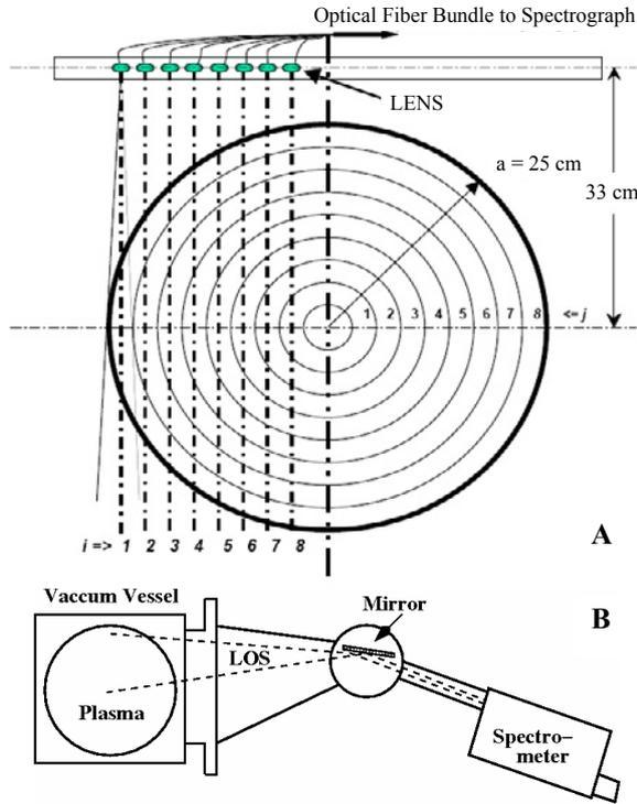
Figure1: Schematic of the viewing geometries of Multi-track Spectrometer (A) and Normal Incidence Spectrometer (B) systems respectively
