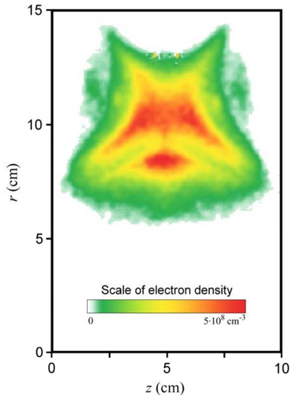
Fig. 3. Distribution of electron density in  $r$ - $z$  plane.
