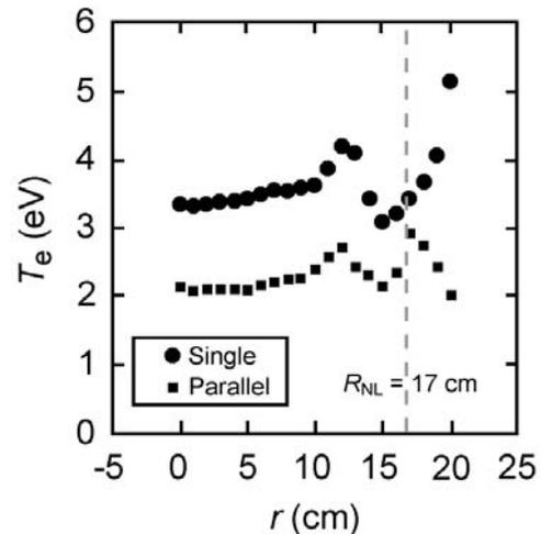
Fig. 6. Radial distribution of the measured electron temperature in NLD plasma using a single turn and parallel turn rf antenna [10]. The operating pressure is about 0.2 Pa (1.5 mTorr), rf is 13.56 MHz and 1 kW.
