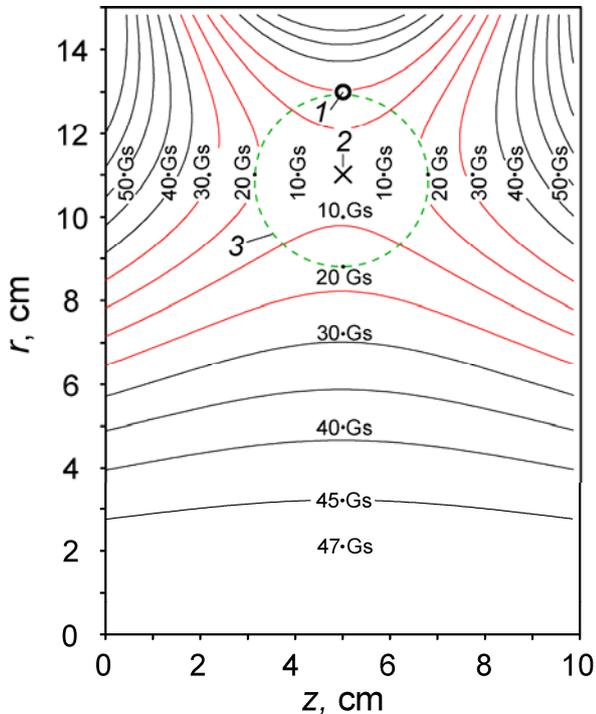
Fig. 2. Magnetic field lines and magnetic field strength in computational domain ( $r$ - $z$  plane). 1 – rf antenna; 2 – position of neutral loop ( $r = 11$  cm and  $z = 5$  cm) and 3 – contour of local ECR. Red lines denote location of the magnetic trap.
