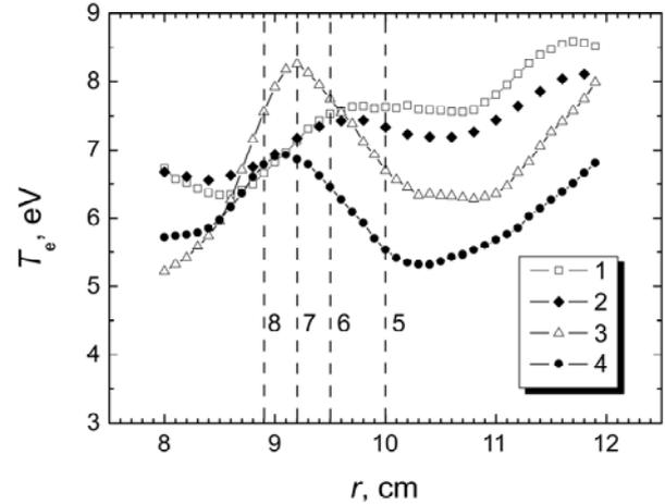
Fig. 5. Radial distribution of the calculated electron temperature as parameters of the frequency and pressure. 1 –  $\omega = 27$  MHz,  $P = 6.6$  mTorr; 2 –  $\omega = 40$  MHz,  $P = 3.3$  mTorr; 3 –  $\omega = 48$  MHz,  $P = 3.3$  mTorr; 4 –  $\omega = 54$  MHz,  $P = 3.3$  mTorr. Lines 5, 6, 7 and 8 denote radius corresponding to the ECR condition at the rf of 27, 40, 48 and 54 MHz, respectively. Radius of neutral loop is 11 cm.
