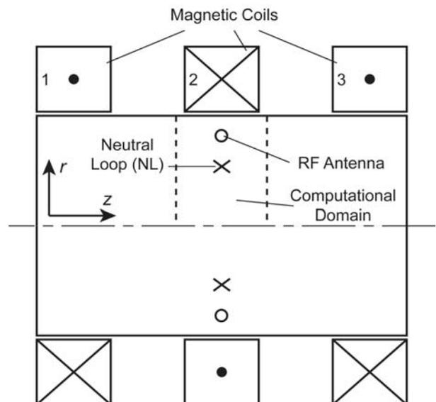
Fig. 1. Schematic diagram of the cylindrical NLD setup. A dashed line denotes computational domain for numerical simulation.
