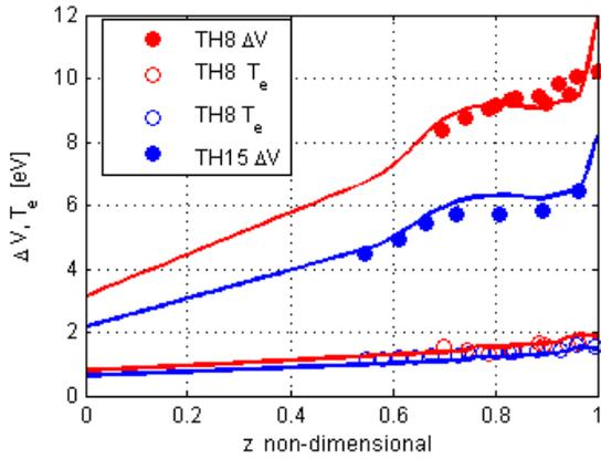
Fig.2 Comparison between calculated and measure plasma parameters for TH8 and TH15
