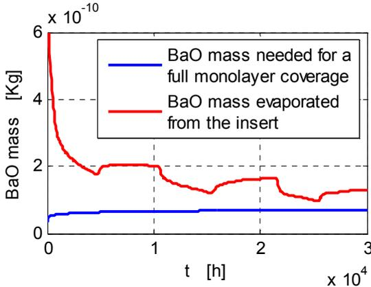
Fig.11 BaO mass needed for a full coverage at startup and evaporated mass during startup T=1150 °C–NSTAR
