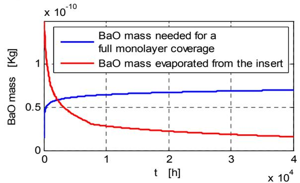
Fig.7 BaO mass needed for a full coverage at startup and evaporated mass during startup  $T_{start}=1100^\circ\text{C}$ – 12A
