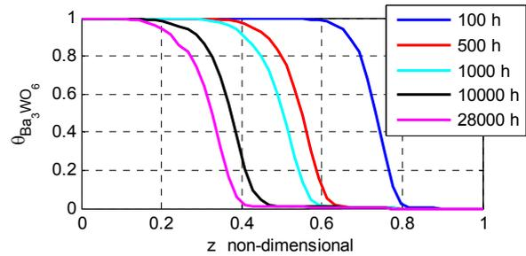
Fig.4 Ba<sub>3</sub>WO<sub>6</sub> surface coverage – 12A
