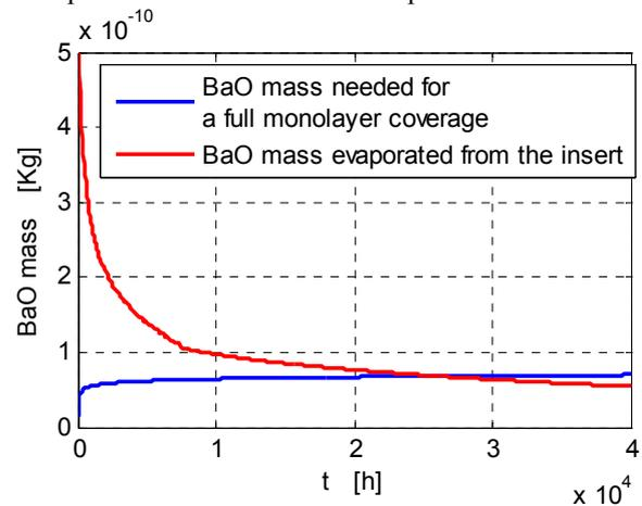
Fig.10 BaO mass needed for a full coverage at startup and evaporated mass during startup T=1150 °C– 12A
