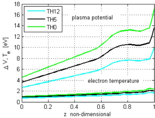
Fig.3 Calculated plasma voltage and temperature profiles for TH12, TH5 and TH0
