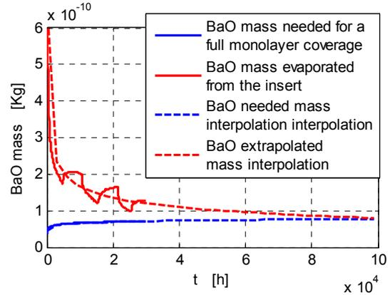
Fig.12 Extrapolation of the deposited and needed BaO mass T=1150 – NSTAR
