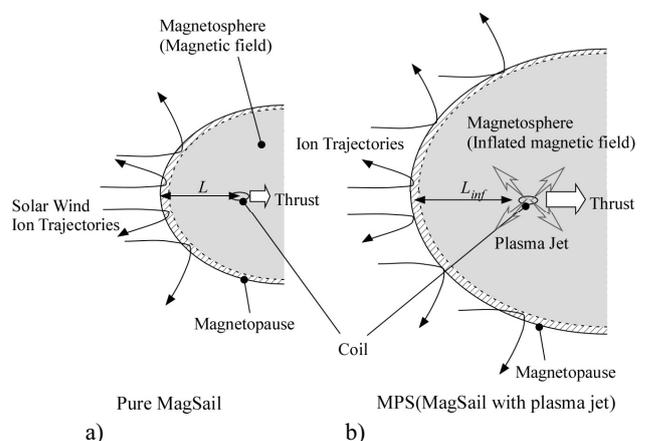
Fig. 1 Concepts of Pure Magnetic Sail and Magnetoplasma Sail.
