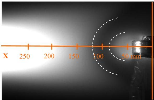
Fig. 4 CCD image of the flow around Pure Magnetic Sail ( $u_{sw}=47$  km/s and  $n_{sw}=1.24 \times 10^{19}$  m<sup>-3</sup>), B-field at Coil center:  $B_S=0.06$  T, without plasma injection.
