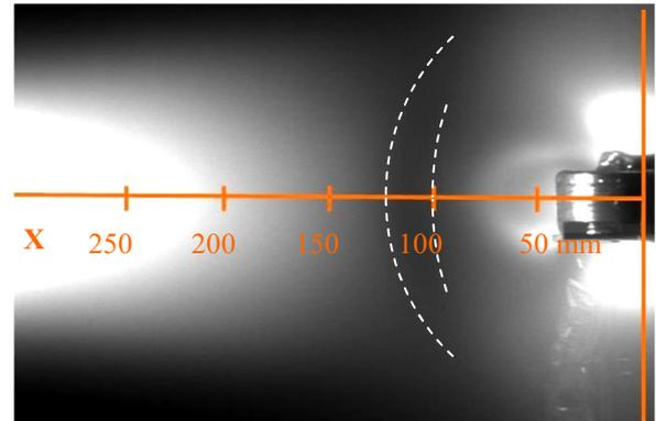
Fig. 5 CCD image of the flow around Magnetoplasma Sail ( $u_{sw}=47$  km/s,  $n_{sw}=1.24 \times 10^{19}$  m<sup>-3</sup>), B-field at Coil center:  $B_S=0.06$  T, with injection plasma ( $u_{inj}=17.2$  km/s and  $n_{inj}=3.2 \times 10^{19}$  m<sup>-3</sup>).
