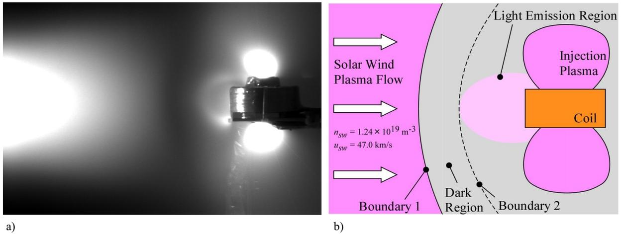
Fig. 3 CCD image of the flow around Magnetoplasma Sail (a) and explanation of the field (b), Solar Wind:  $u_{sw}=47$  km/s,  $n_{sw}=1.24 \times 10^{19}$  m<sup>-3</sup>, Coil:  $B_S=0.06$  T, Injection plasma:  $u_{inj}=17.2$  km/s,  $n_{inj}=3.2 \times 10^{19}$  m<sup>-3</sup>.
