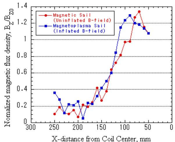
Fig. 6 Magnetic flux density ( $B_z$ ) of Pure MagSail and Magnetoplasma Sail along the X-axis;  $B_z$  was normalized by the magnetic field without the interaction with the solar wind ( $B_{z0}$ ).
