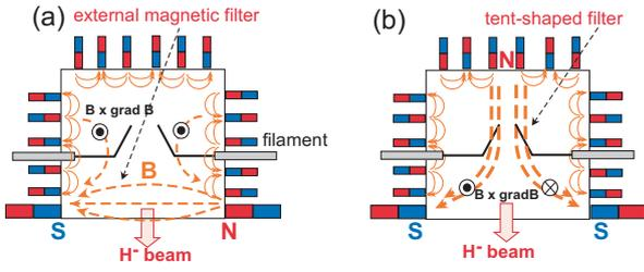
Fig.3 Schematics of two magnetic field configurations; (a) the original external filter and (b) tent-shaped filter.
