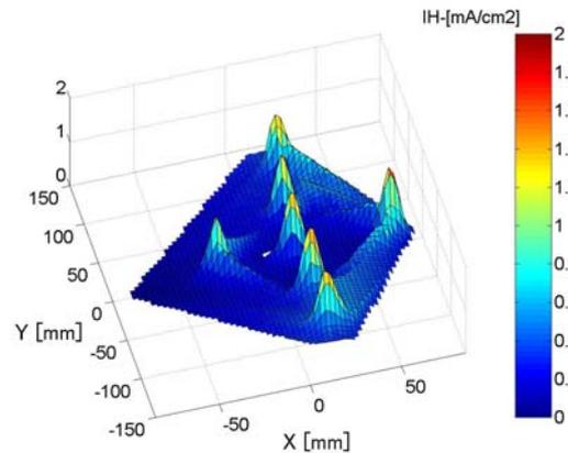
Fig.6 The surface plot of beam intensities of beamlets extracted from seven apertures.
