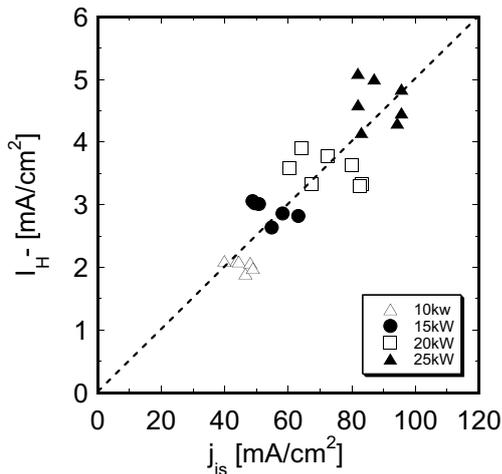
Fig.7 A correlation between the incident flux represented by positive ion flux at several positions in the longitudinal direction and the local beam current density at corresponding positions.
