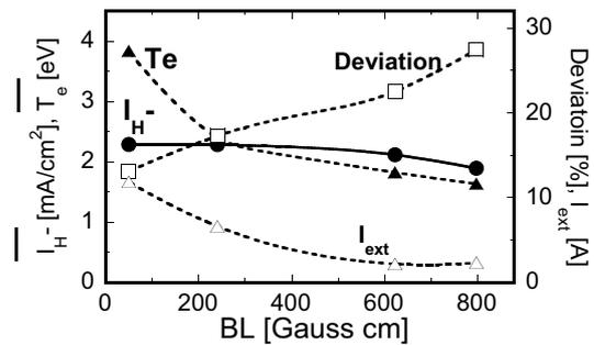
Fig.2 Dependence of averaged values over the extraction area of  $I_{H^-}$  (closed circles),  $T_e$  (closed triangles), deviation (open squares) and  $I_{ext}$  (open triangles) on the magnetic filter strength.
