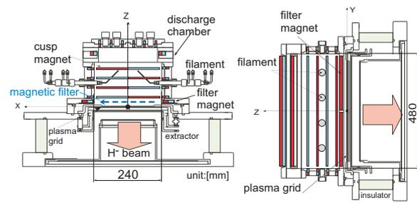
Fig.1 Schematic of the JAEA 10 ampere negative ion source figure.
