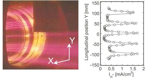
Fig.5 (left) A snapshot of the uniform  $H^-$  ion beam extraction with a small divergence angle in the tent filter, (right) the beam intensity profiles of longitudinally distributed five beamlets. In this photograph, beamlets extracted from peripheral apertures also appeared.
