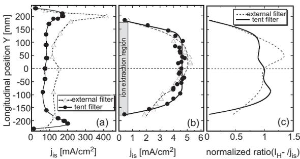
Fig.4 Comparison of longitudinal distributions of (a) ion saturation current density, (b)  $I_{H^-}$  and (c) their normalized ratio in the tent filter (closed circles) and the external filter (open triangles), respectively.
