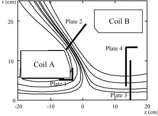
Fig. 2 Example of field lines of slanted cusp magnetic field.
