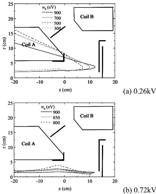
Fig. 6 Examples of ion orbit calculation for two-stage deceleration.  $I_{AC} = 22.5\text{A}$  and  $I_B = 20\text{A}$  and  $V_{34} = 1\text{kV}$ . Here, (a) and (b) are for  $V_1 = 0.26\text{kV}$  and  $0.72\text{kV}$ .
