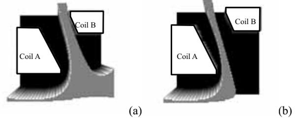
Fig. 3 Examples of movable region for an electron of 2keV. Plate3 and Plate4 are biased with 1kV, and  $I_{AC} = 30A$ , and  $I_B = 10A$  and  $20A$  for (a) and (b), respectively.
