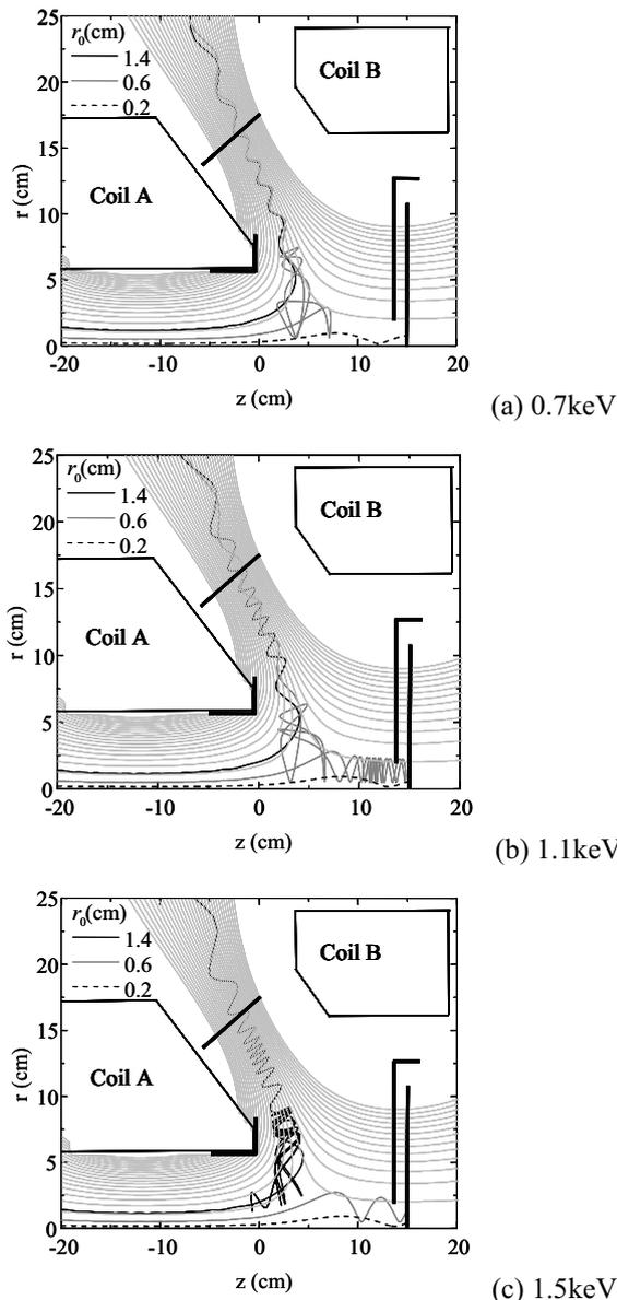
Fig. 4 Examples of electron orbit calculation.  $I_{AC} = 30A$  and  $I_B = 20A$  and  $V_{34} = 1kV$ . Energy of incident electrons is 0.7, 1.1, and 1.5keV for (a), (b), and (c), respectively.
