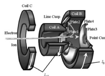
Fig. 1 CUSP-DEC experimental device.
