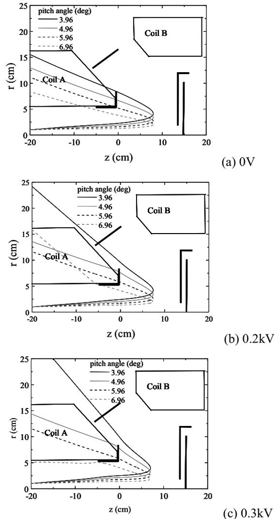
Fig. 5 Examples of ion orbit calculation.  $I_{AC} = 30A$  and  $I_B = 20A$  and  $V_{34} = 1kV$ . Energy of ion is 0.5keV and incident position is  $(r, z) = (1cm, -20cm)$ .  $V_1$  is 0, 0.2, and 0.3kV for (a), (b), and (c), respectively.
