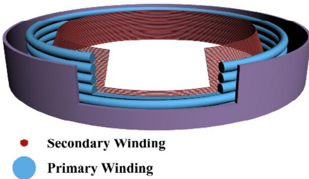
Fig.1 Typical configuration of a tesla transformer
