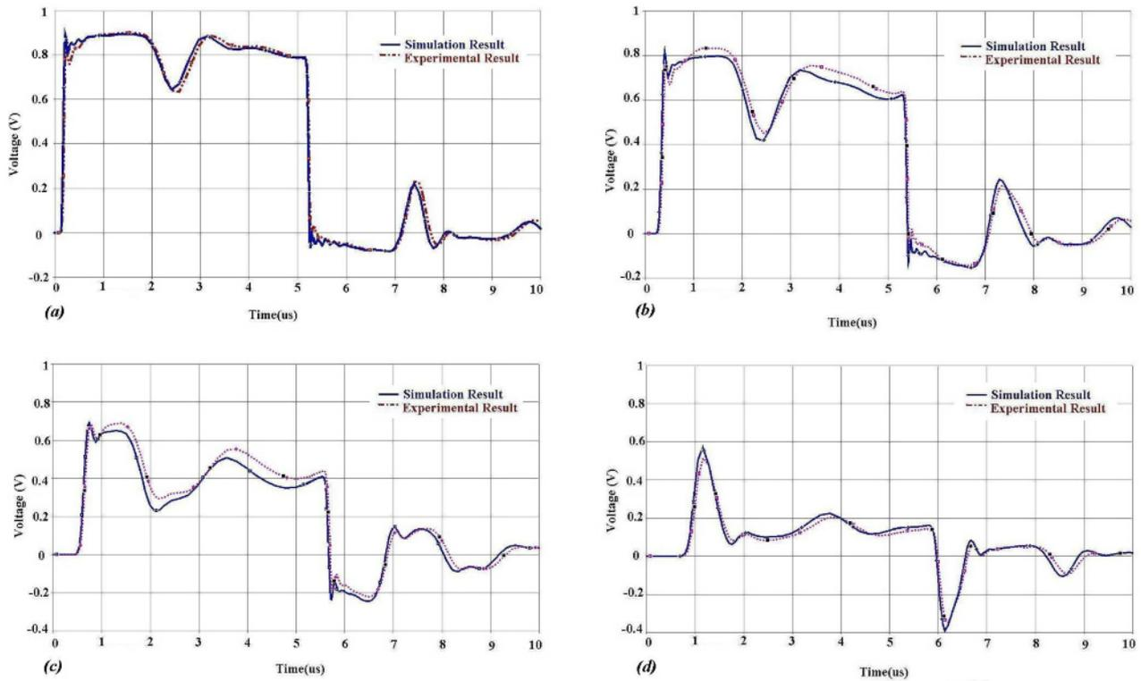
Fig.4 Comparison between numerical and measured values. Voltage to ground of turn 30, 24, 13 and 7
