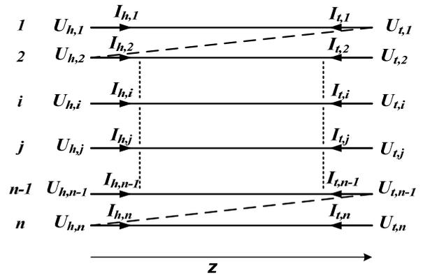
Fig.2 MTL model of the tapered secondary winding.
