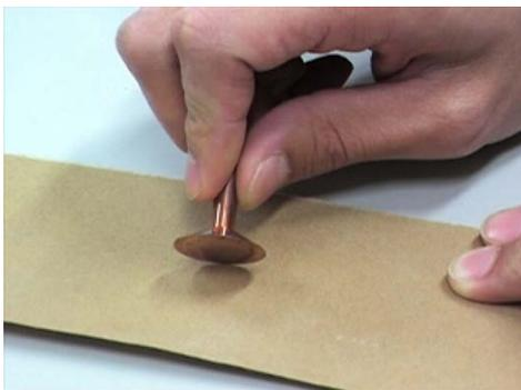
Fig.7 Rasp of the emission edge of disk cathode.
