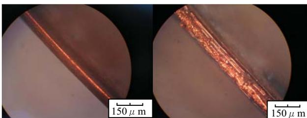
Fig.8 Micrograph of the emission surfaces. Left-side is the mirror finished copper cathode and right-side is the corresponding surface after scratching by sandpaper.
