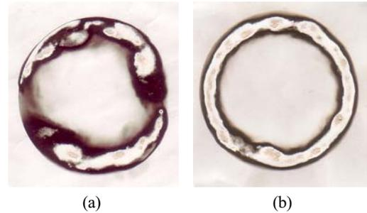
Fig.6 Burn patterns of electron beam for the mirror finished cathode made of copper: (a) is obtained with the mirror-like surface and (b) is after rasing the surface. Both are obtained by 1-shot without velvet. Beam voltage is about 90 kV. Beam current is about 400 A for (a) and about 450 A for (b).
