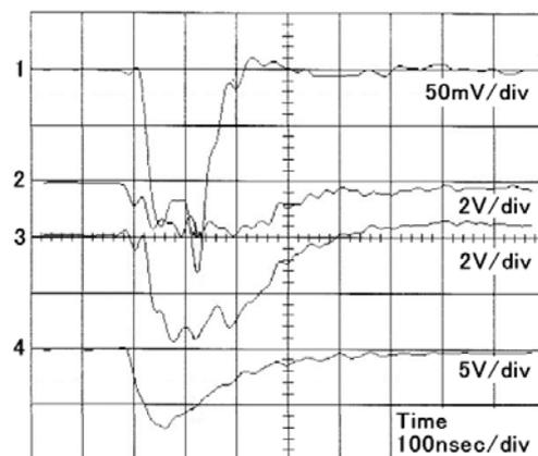
Fig. 11 An example of long-pulse operation: 1 microcathode voltage, 2 cathode current, 3 beam current and 4 beam voltage. Peak values of beam voltage and beam current are about 90 kV and 400 A, respectively. Estimated microwave power level is around 100 kW.
