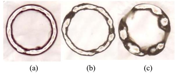
Fig.9 Burn patterns of (a) copper, (b) stainless steel and (c) aluminum disk cathode. They are obtained by 1-shot without velvet. Beam voltage is about 90 kV. Beam currents are around 400 A.
