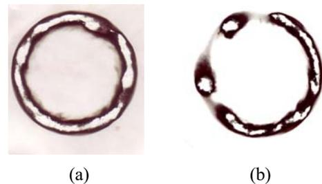
Fig.10 Burn patterns of (a) copper and (b) stainless steel disk cathode. They are obtained by 1-shot without velvet. Beam voltage is about 60 kV. Beam current is about 270 A for (a) and about 190 A for (b).
