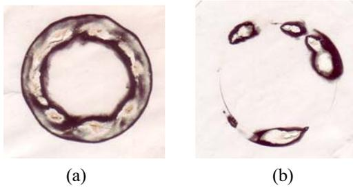
Fig.3 Burn patterns of 5-shot overlay for the tubular cold cathode made of aluminum at about 90 kV, (a) with velvet and (b) without velvet. The beam current is about 350 A with velvet and 100 A without velvet.
