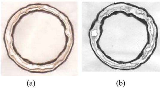
Fig.4 Burn patterns of 5-shot overlay, (a) for the solid disk cone made of stainless steel and (b) for the conical shell made of stainless steel. Both are obtained without velvet at about 90 kV and 450 A.
