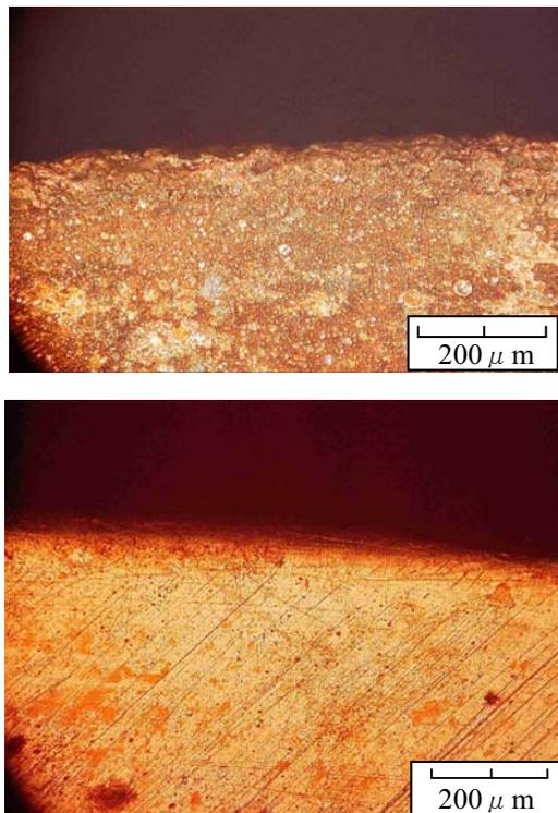
Fig.5 Micrograph of the surfaces of the lathe finished copper cathode (top) and mirror finished copper cathode (bottom).
