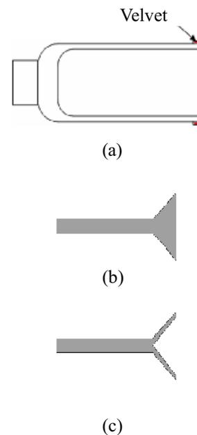
Fig.2 Cross section of (a) tubular, (b) disk and (c) conical shell cathodes.
