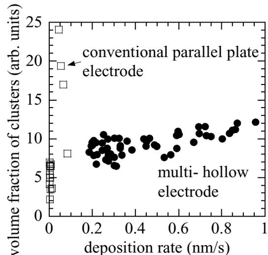
Fig. 7. Dependence of volume fraction of clusters on deposition rate for the multi-hollow electrode (solid circles) and the conventional parallel plate electrode (open squares). Experimental conditions are the same as those of Fig. 4.
