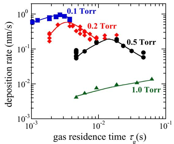
Fig. 4. Dependence of deposition rate on gas velocity as a parameter of pressure. Conditions:  $\text{SiH}_4$  100%, 60MHz, 150Vpp, substrate temperature  $100^\circ\text{C}$ .
