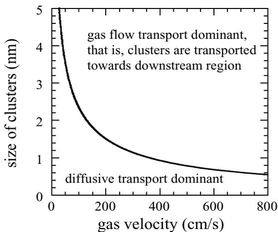
Fig. 3. Dependence of lower limit size of gas flow transport dominant region on gas velocity for  $p=0.2\text{Torr}$ ,  $T=100^\circ\text{C}$ .
