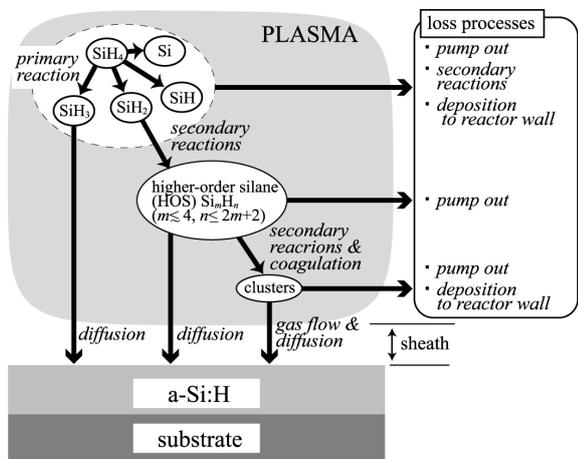
Fig. 1. A model of main reactions in silane plasma.
