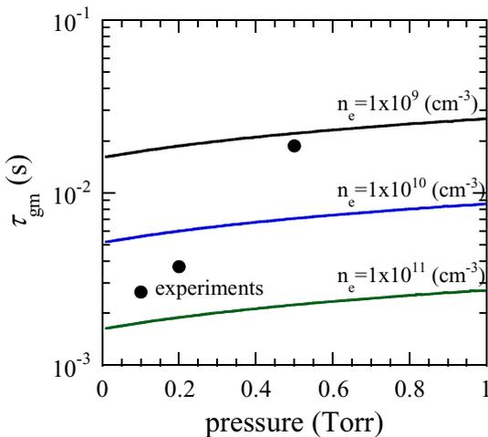
Fig. 5. Dependence of  $\tau_{gm}$  on pressure. Solid circles indicate experimental results. Line shows the theoretical curve.
