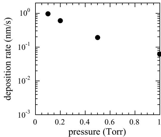
Fig. 6. Dependence of the maximum deposition rate for each pressure on pressure.
