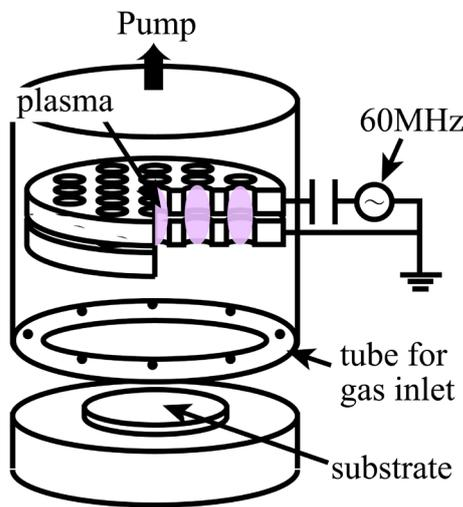
Fig. 2. Multi-hollow discharge plasma CVD reactor.
