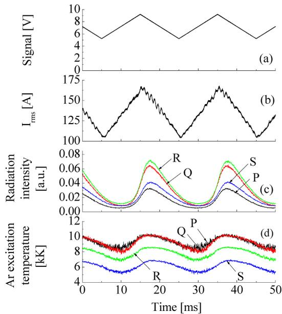
Fig. 7 Time evolution in (a) modulation signal, (b) the inverter output current in root-mean-square value, (c) radiation intensity of the Ar atomic line at 714 nm, (d) Ar excitation temperature from the two-line method. The coil current amplitude is modulated into a triangular waveform.
