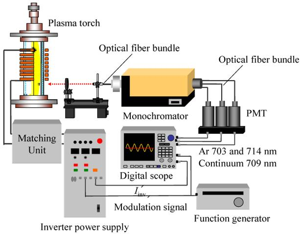
Fig. 4 Spectroscopic observation system.
