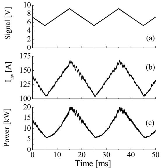
Fig. 5 Time evolution in (a) modulation signal, (b) the inverter output current in root-mean-square value, (c) Inverter output effective power. The coil current amplitude is modulated into a triangular waveform.
