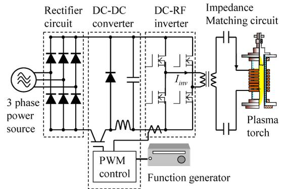
Fig. 2 Electric circuit for AMITP system.
