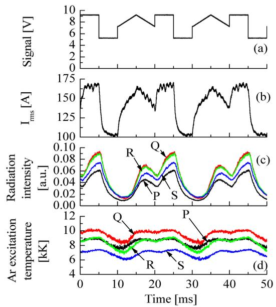
Fig. 8 Time evolution in (a) modulation signal, (b) the inverter output current in root-mean-square value, (c) radiation intensity of the Ar atomic line at 714 nm, (d) Ar excitation temperature from the two-line method. The coil current amplitude is modulated into a triangle-rectangular waveform.
