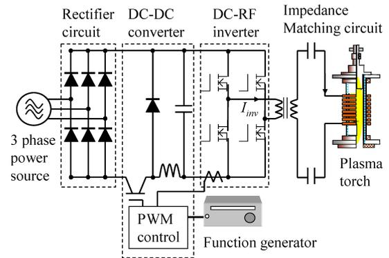
Fig. 2 Electric circuit for AMITP system.
