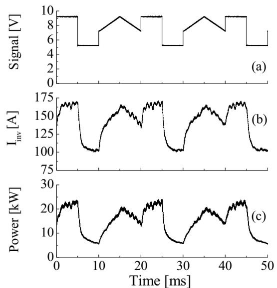
Fig. 6 Time evolution in (a) modulation signal, (b) the inverter output current in root-mean-square value, (c) Inverter output effective power. The coil current amplitude is modulated into a triangle-rectangular waveform.
