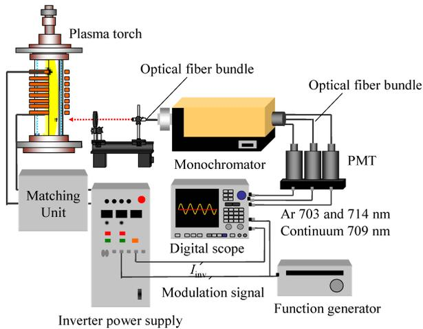
Fig. 4 Spectroscopic observation system.
