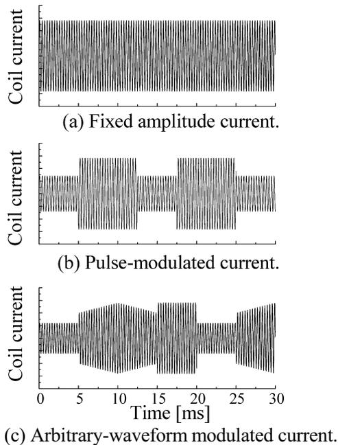
Fig. 1 Concept of modulated coil current
