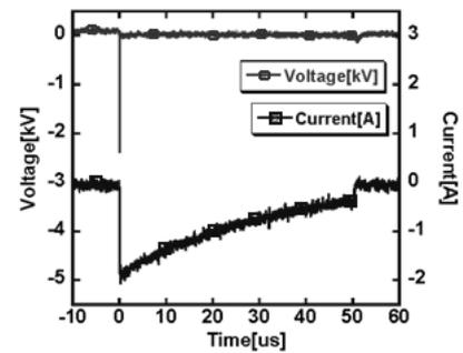
Fig.14 Voltage and current waveforms of microplasma jet reactor without BJTs at output.
