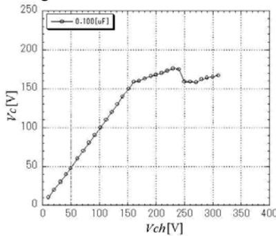
Fig.2 Dependence of  $V_c$  on  $V_{ch}$  (2SC2655).
