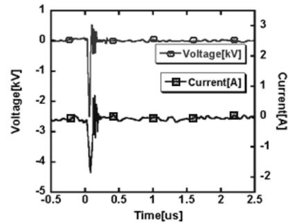
Fig.13 Voltage and current waveforms of microplasma jet reactor with BJTs at output.
