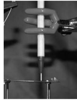
Fig.11 Photograph of microplasma jet reactor.
