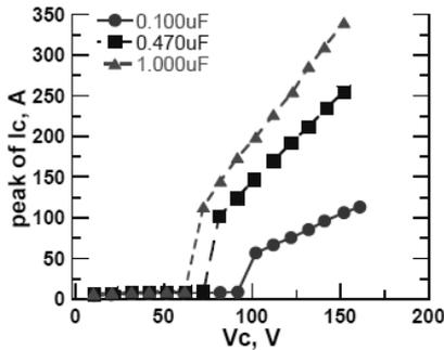
Fig.5 Current and voltage characteristics for different capacitance.
