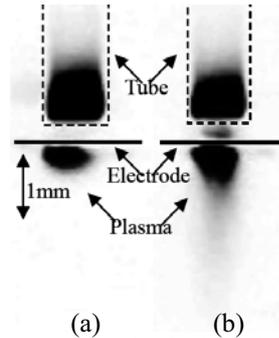
Fig.12 Photograph of microplasma jet.
