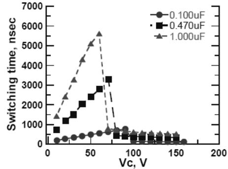
Fig.7 Dependence of switching time on  $V_c$  for different capacitance.
