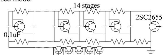
Fig.9 Schematic circuit diagram of Miniaturized Marx generator.
