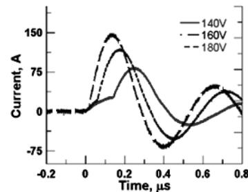
Fig.4 Collector current waveforms for three different  $V_{ch}$ . (2SC5000,  $C=0.100\mu\text{F}$ ).
