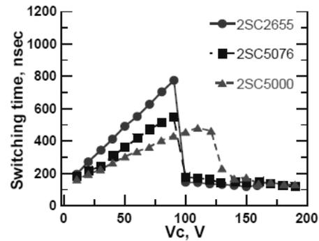
Fig.8 Dependence of switching time on  $V_c$  for different BJTs.
