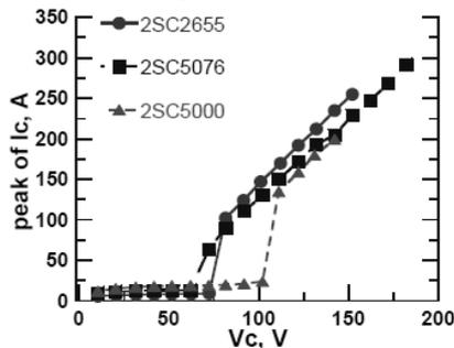
Fig.6 Current and voltage characteristics for different BJTs.
