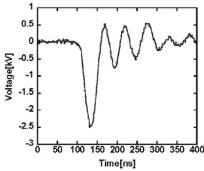
Fig.10 Output voltage of Miniaturized Marx generator.
