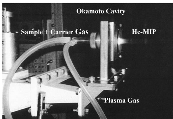
Fig.2. Photograph of the He-MIP at atmospheric pressure generated by the Okamoto Cavity with aqueous fluoride, NaF nebulization. Microwave power = 600 watt, plasma and carrier gas flow rate  $G_p = 10.5$  l/min and  $G_c = 0.3$  l/min, respectively [5].
