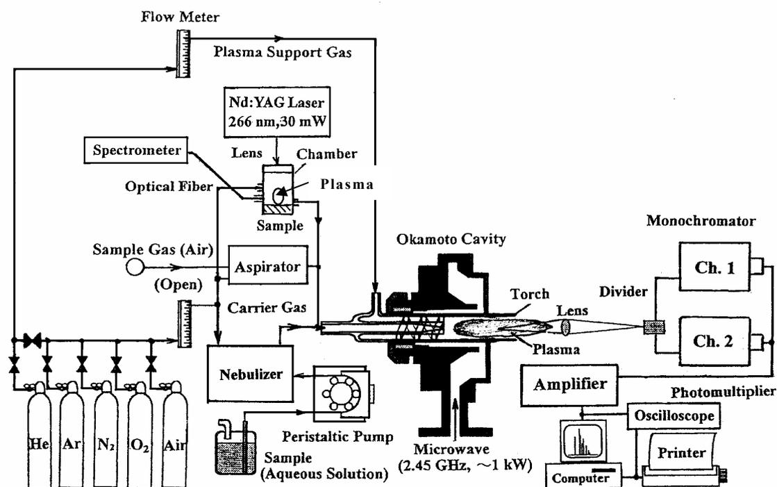
Fig.1. Experimental setup of the laser-ablation / helium microwave-induced plasma atomic emission spectrometry (LA/He MIP AES) for the particle analysis.
