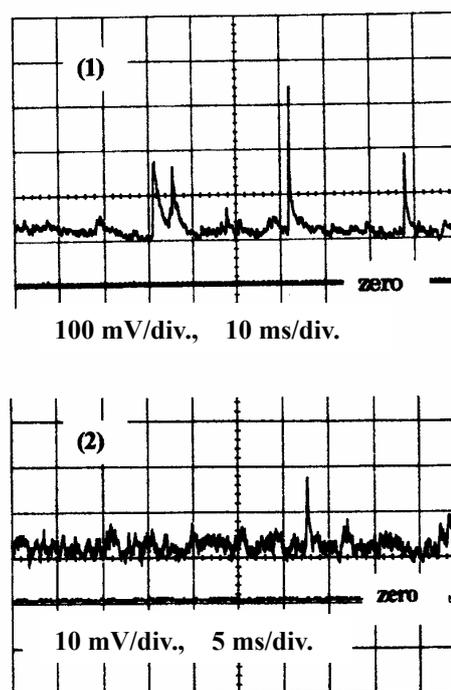
Fig.5. Sample output (1) Al I(396.2 nm) and (2) C I(247.9 nm) emission obtained when aluminum plate was ablated by the laser.
