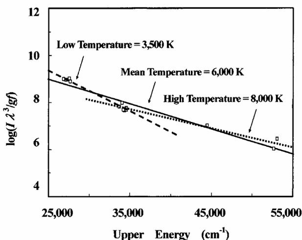
Fig.3. Boltzmann plot for Fe I upper levels with He-MIP. Microwave power is 800 watt.
