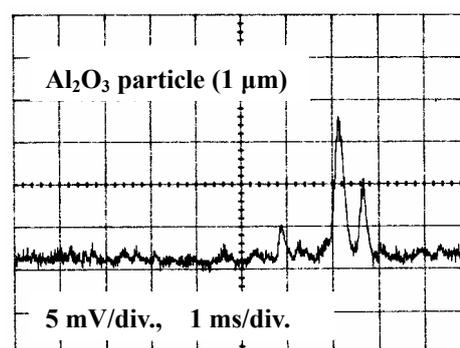
Fig.6. Temporal behavior of Al (396.2 nm) emission from the  $\text{Al}_2\text{O}_3$  particle.
