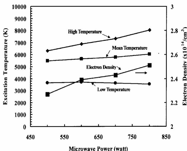
Fig.4. Effects of microwave power on the excitation temperature and the electron density.
