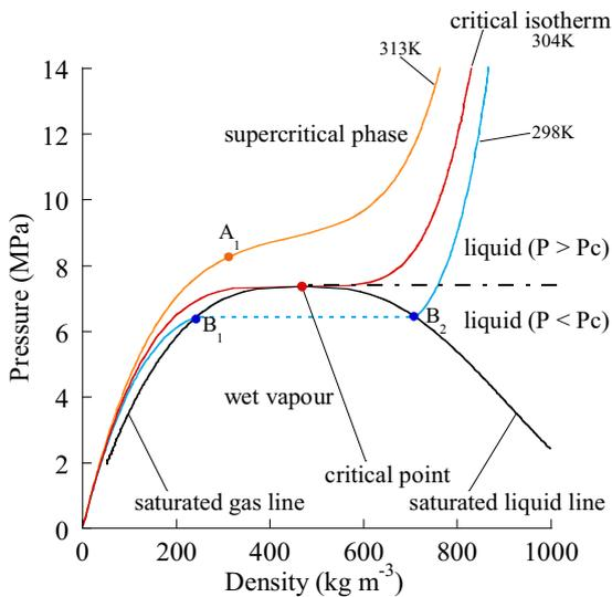
Fig. 1. CO<sub>2</sub> pressure-density diagram
