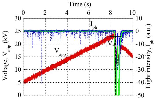
Fig. 3b. Typical positive corona onset and breakdown voltages in supercritical phase at 313 K
