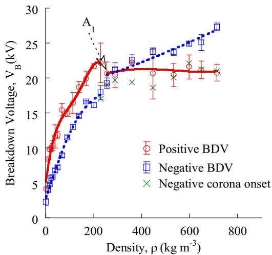
Fig. 4a. Dependence of BDV on CO<sub>2</sub> density;
