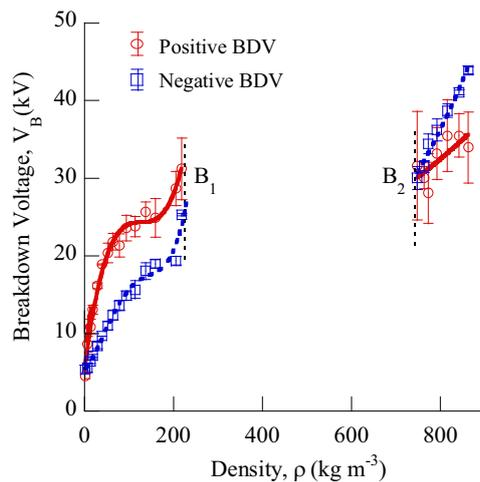
Fig. 4b. Dependence of BDV on CO<sub>2</sub> density;
