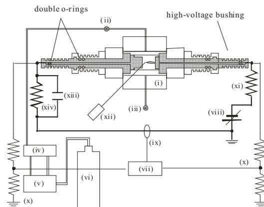
Fig. 2. Schematic diagram of the experimental setup: (i) test cell, (ii) CO<sub>2</sub> inlet, (iii) CO<sub>2</sub> outlet, (iv) syringe pump, (v) cooling system, (vi) CO<sub>2</sub> container, (vii) digital oscilloscope, (viii) dc power source, (ix) current transformer, (x) high voltage probe, (xi) damping resistor, 2 MΩ (xii) photomultiplier (xiii) capacitor, 17x10<sup>-3</sup> μF and (xiv) damping resistor, 2 MΩ
