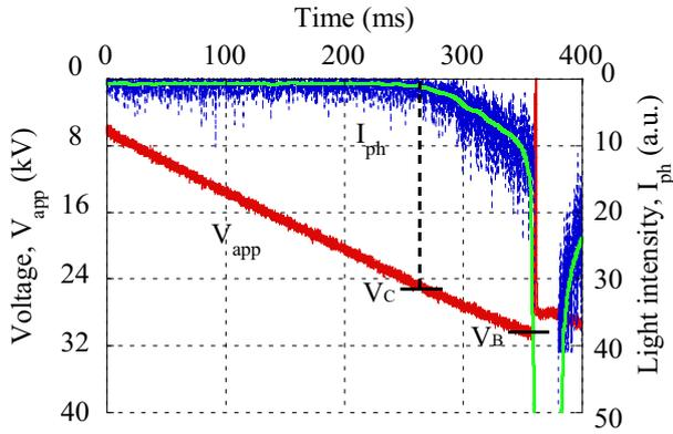
Fig. 3a. Typical negative corona onset and breakdown voltages in supercritical phase at 313 K
