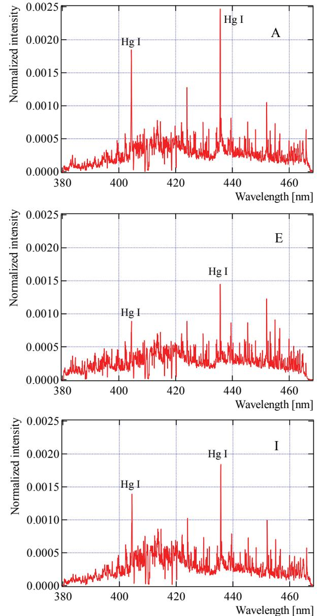
Fig. 5 Optical emission spectra taken at lamp locations indicated by A (tube bottom), E (tube center), and I (tube top) in Fig. 4.
