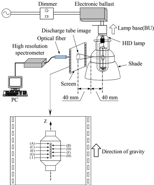
Fig. 4 Schematic diagram of the experimental setup for measuring spatial distributions of OES. Points A through I indicate the positions where the inlet of the optical fiber connected to the spectrometer was located.
