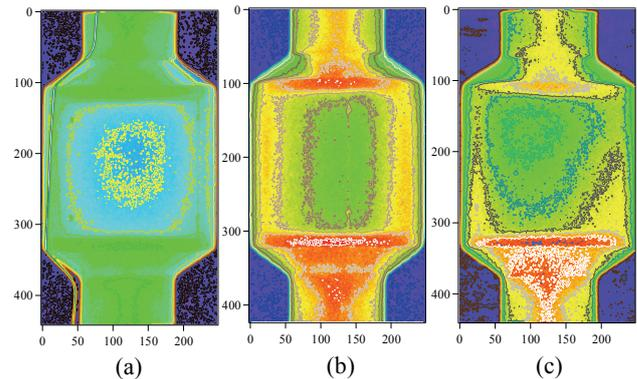
Fig. 2 Absorption of discharge tubes indicated by color. Dark blue or black indicates 0% absorption, and the absorption is larger from green to red. (a) as-received lamp, (b) sample A, and (c) sample B.
