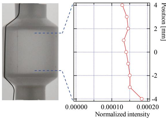
Fig. 7 Spatial distribution of line spectrum emission of Dy at 421.18 nm.
