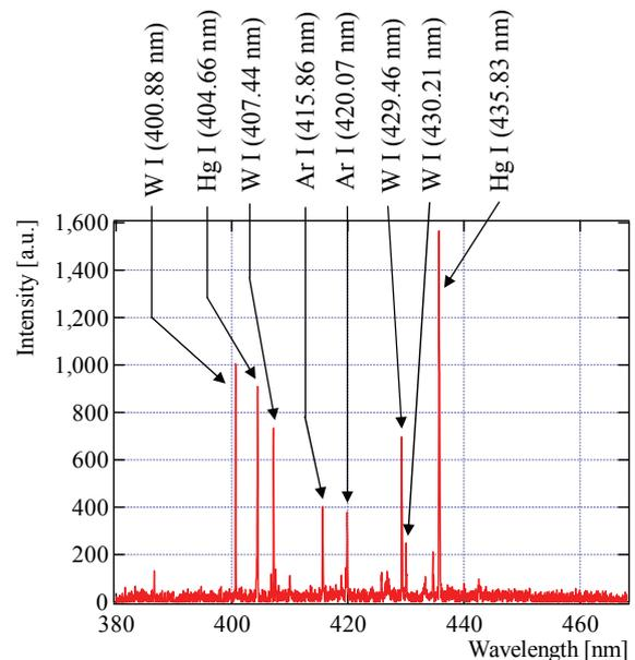
Fig. 3 Optical spectrum of light from HID plasma during lamp ignition. (About 100 ms from the ignition.)
