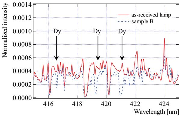
Fig. 6 The optical emission and absorption of Dy.
