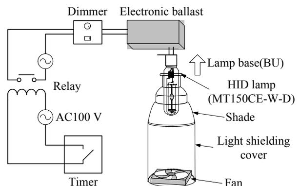
Fig. 1 Schematic diagram of the experimental setup for short duration turn-on/turn-off operation.
