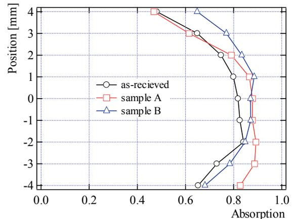
Fig. 8 Absorption by Al spectral line at 394.40 nm plotted as functions of vertical position for as received sample, sample A, and sample B.
