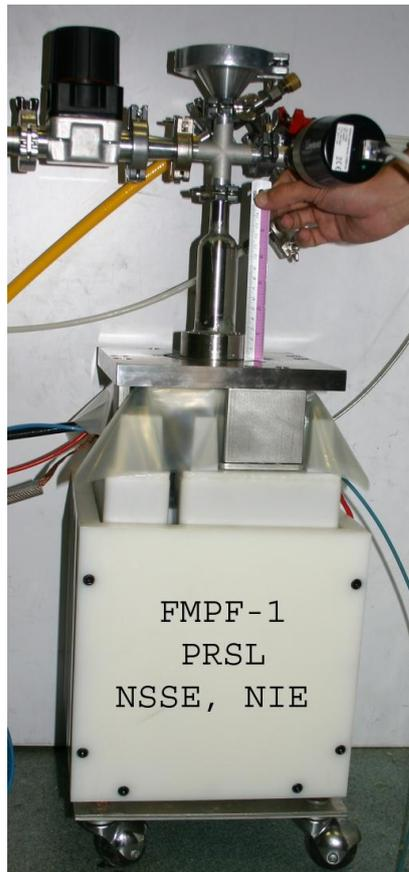
Fig.1 The 'FMPF-1' Miniature PF Device.
