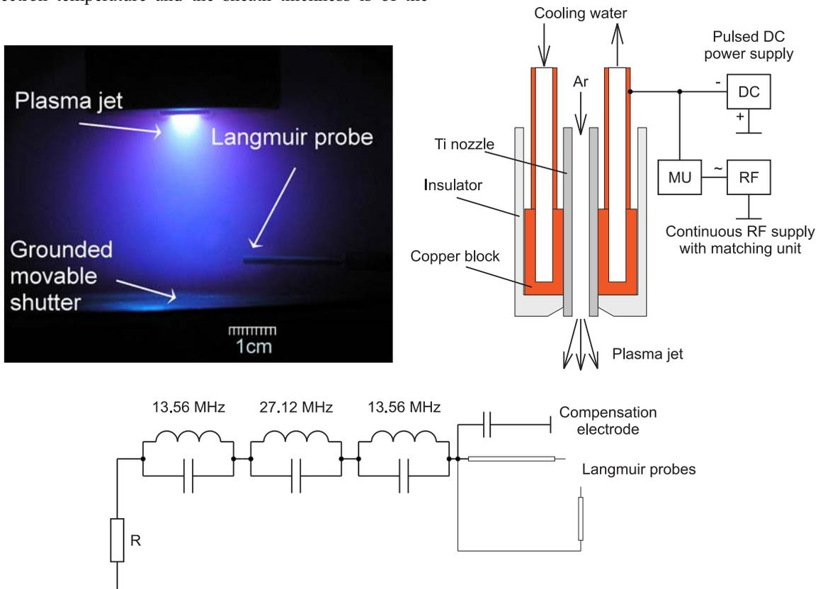
**Fig. 1.** The schematic diagram of the low-pressure plasma jet system. Only the plasma nozzle located at the axis of the grounded cylindrical vacuum vessel with the diameter of 300 mm is shown. In the top left corner a photo of a typical discharge is introduced. The details on the system and experimental conditions are given in the text.
