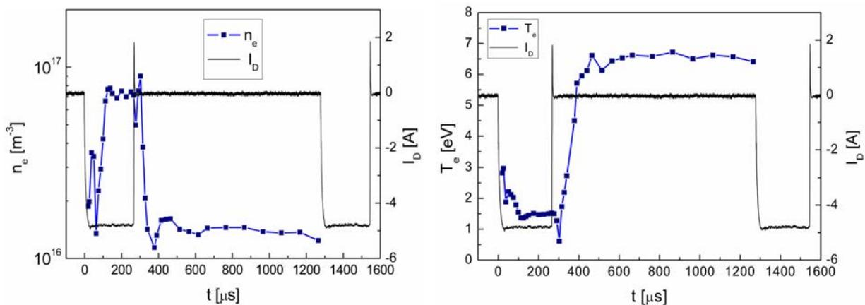
**Fig. 3.** The temporal dependences of electron density (left panel) and of electron temperature (right panel) in the DC-powered single plasma jet system in pulsed regime in argon. Ti nozzle diameter 6mm, pressure 3.5 Pa, argon flow 110 sccm,  $h=20$  mm. Repetition rate 575 Hz, duty cycle 0.175, active pulse length 270  $\mu\text{s}$ . Discharge current during the active part of the period 5 A. The plasma parameters in the idle part of the period correspond to the background RF plasma.
