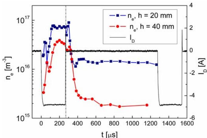
**Fig. 5** The temporal dependences of electron density in the DC-powered single plasma jet system in pulsed regime in argon at two different distances from the nozzle exit. The experimental conditions are the same as that in Fig. 3.
