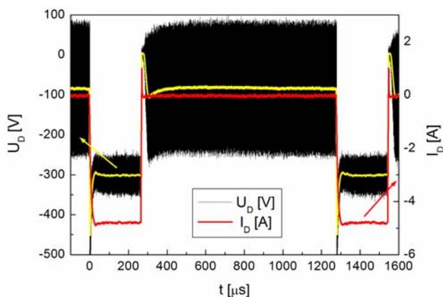
**Fig. 4** The temporal dependences of DC discharge voltage and discharge current. The superimposed CW RF voltage is also shown. The experimental conditions are the same as that in Fig. 3.
