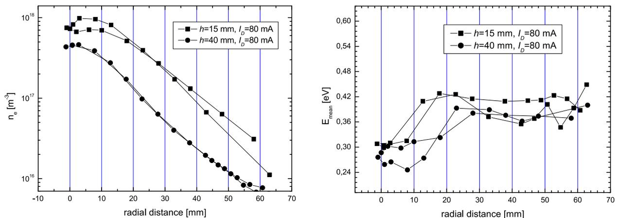
**Fig. 2.** The radial dependences of electron density (left panel) and of electron mean energy (right panel) in the DC-powered single plasma jet system. Ti nozzle diameter 6 mm, pressure 20 Pa, argon flow 30 sccm.
