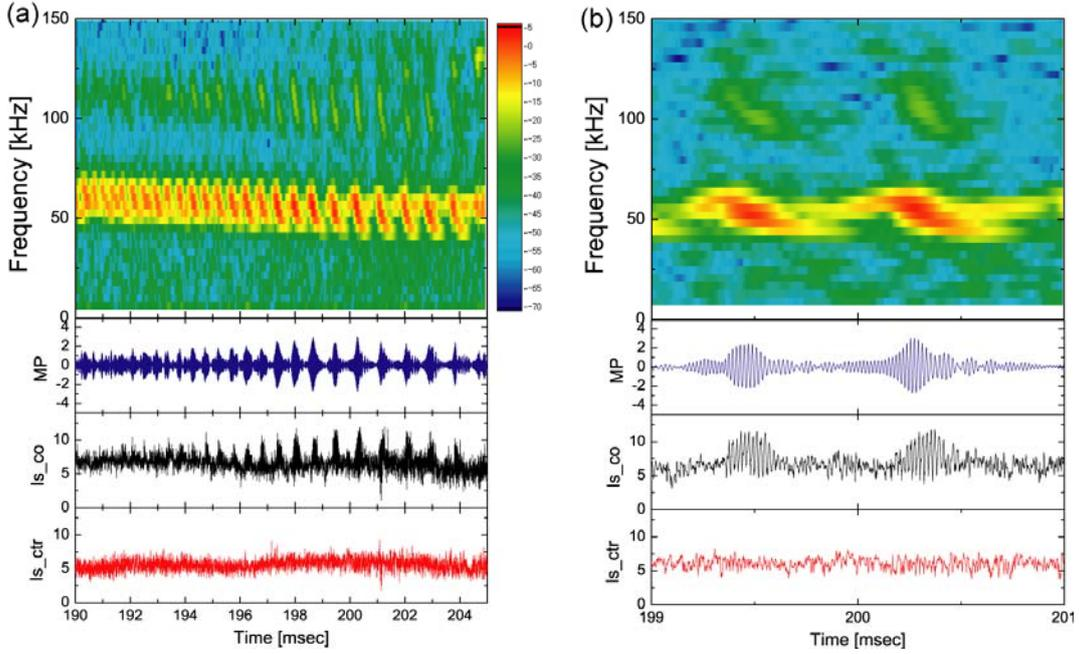
Fig.2 (a) The contour map of the power spectrum of magnetic fluctuation (running FFT with time window of 0.256 msec) and the wave forms of Mirnov signal (MP) located on the chamber wall, co-directed ( $I_{s\_co}$ ) and ctr-directed ( $I_{s\_ctr}$ ) ion currents measured by the HDLP at  $r/a=0.9$ . (Shot No. 30013). (b) The enlarged figure of (a).
