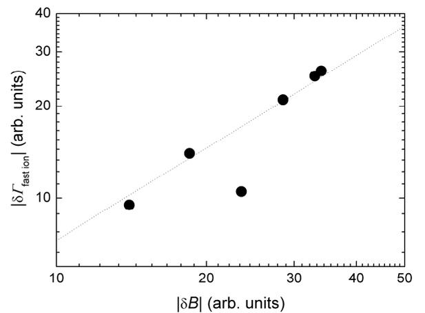
Fig.3 The amplitude of fast ion flux as a function of GAE amplitude measured at the chamber wall. The dashed line indicates the  $s=1$  line in the function of  $\delta \Gamma_{\text{fast\_ion}} \propto \delta B^s$ .
