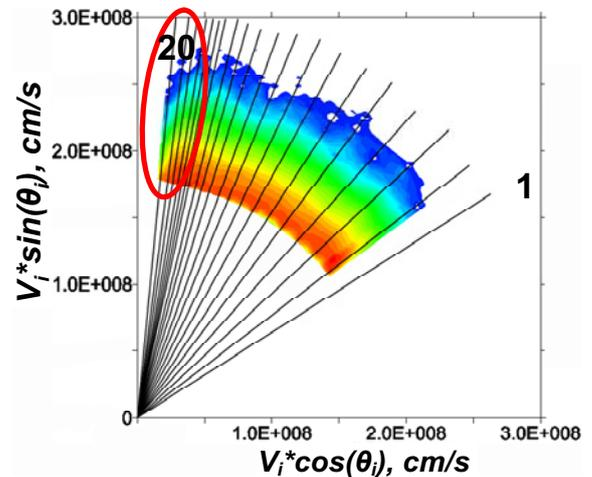
Fig.5 Experimental result of angular distribution of fast particles for  $R_{ax}=3.6m$  obtained by ARMS-T during operation of the perpendicular NBI#4.
