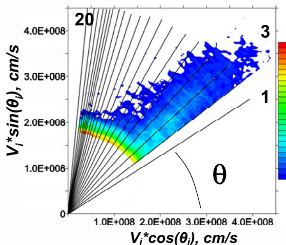
Fig.4 Energy spectrum measured along 19 sightlines ( $i$  is index of the sightline,  $\theta$  is the angle between the sightline and magnetic axis).
