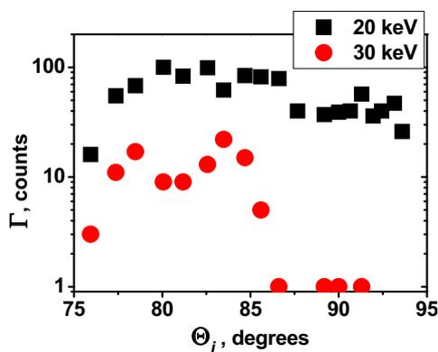
Fig.7 Angular distribution of 20keV(black squares) and 30keV (red circles) protons. ( $i$  is index of the sightline,  $\theta$  is the angle between the sightline and magnetic axis).
