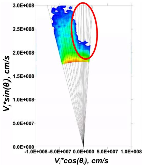
Fig.6 Experimental result of angular distribution of fast particles for  $R_{ax}=3.6m$  obtained by ARMS-P during operation of the perpendicular NBI4.
