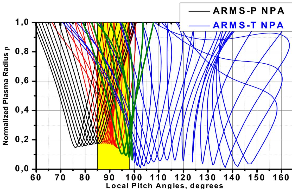
Fig.1 The sheaf of pitch-angles along the sightlines of ARMS-T NPA (blue and green colors) and of ARMS-P NPA (black and red colors)
