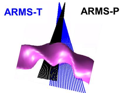
Fig.2 Top view of ARMS-T and ARMS-P diagnostic sightlines versus LHD plasma column.
