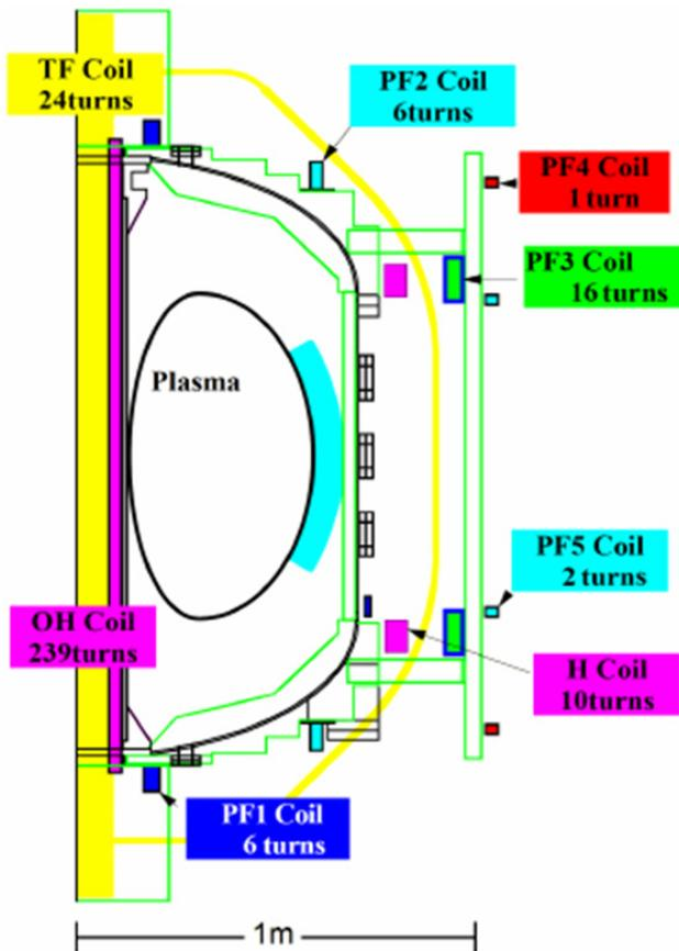
Fig. 1 Cross section of TST-2 and poloidal coils. In this experiment, the vertical field is generated by the PF1 and PF2 coils connected in series. Only PF1, PF2 and TF coils were used. In the discharge shown in Fig. 6, the PF1 coil was operated with 9 turns.
