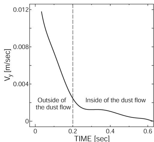
Fig. 3. Temporal variation of perpendicular velocity  $v_y$  of the dusts which enter from the outside into the counter stream. Ar flow rate is 0.5 sccm.
