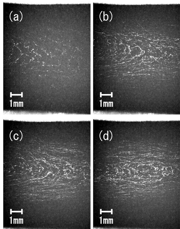
Fig. 5. Dependences of flow patterns on flow rate of Ar gas. (1) 0.1 sccm, (b) 0.2 sccm, (c) 0.3 sccm, (d) 0.4 sccm. RF power is 4 W.
