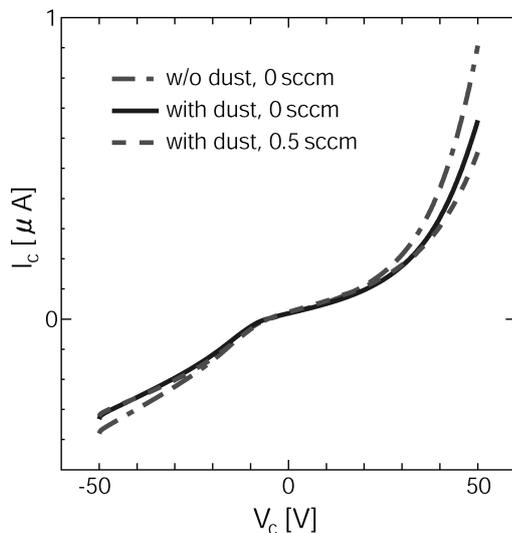
Fig. 4. Collector  $V_c - I_c$  curve with and without dusts and neutral gas flow.
