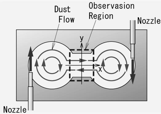
Fig. 2. Observation region of counter stream above a dumbbell-shape levitation electrode.
