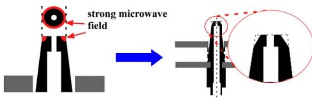
Fig.8 Moderation of localized electric field by cutting the sharp edge of TIAGO nozzle head.
