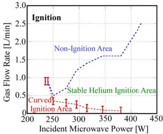
Fig.5 Ignition area for straight helium discharge in the parameter space of helium gas flow rate at atmospheric pressure and incident microwave power. The area between the two boundaries corresponds to straight helium discharge ignition. The upper line shows the boundary for straight discharge ignition above which we do not have any initial ignition, while the lower line does the boundary for curved discharge, below which we have rotating curved discharge ignition.
