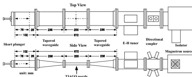
Fig.1 Microwave circuit for plasma torch at atmospheric pressure.
