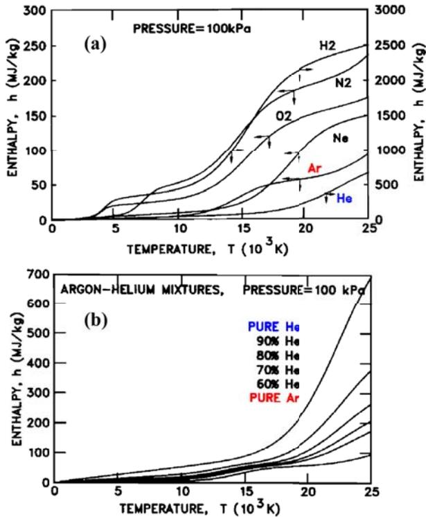
Fig. 6 Enthalpy for various gases. (a) Specific enthalpy of various gases at atmospheric pressure versus temperature. (b) Specific enthalpy of various Ar-He mixtures (vol %) at atmospheric pressure versus temperature. The upper most line corresponds to pure helium From Figs. 6.16 and 6.19 of ref [5].
