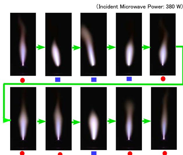
Fig.9 Smooth transitions from one to the other by changing the helium gas flow rate in the case of modified TIAGO nozzle shown in Fig.8. The circle corresponds to normal straight discharge, while the square curved one.
