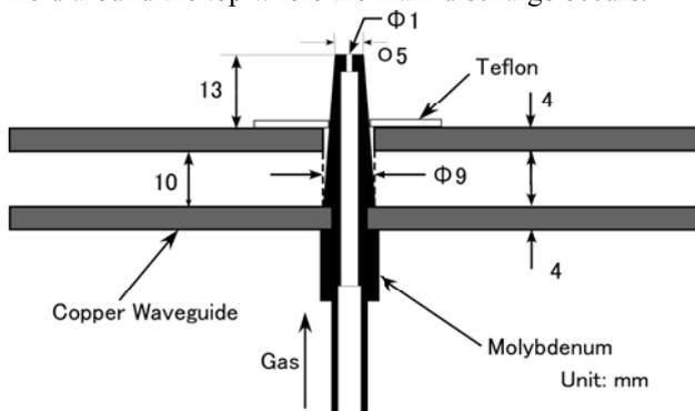
Fig.2 TIAGO nozzle set on the straight waveguide for microwave-sustained plasma torch.
