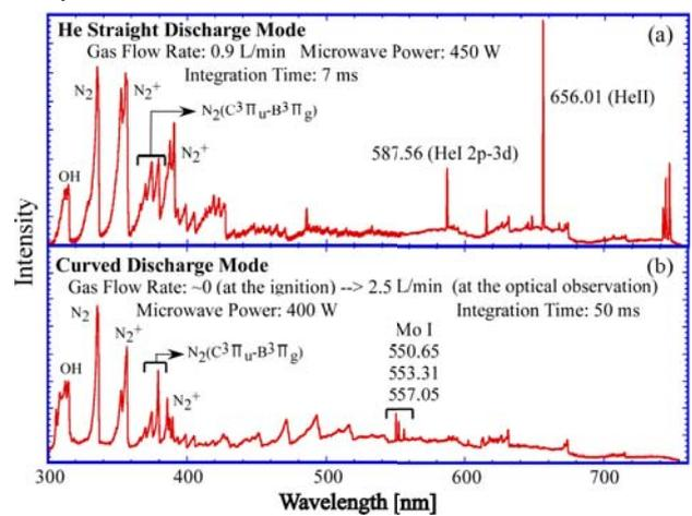
Fig.4 Spectra of optical emission from the foot of jet plasma close to the nozzle head. (a) was obtained from the straight helium plasma jet, while (b) corresponds to the curved discharge mode
