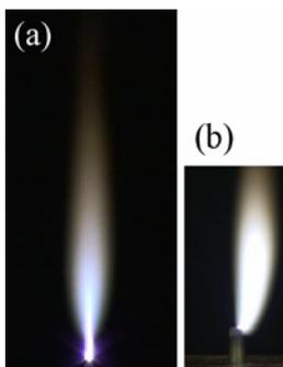
Fig.3 Typical still photos of microwave-sustained plasma torch (a) straight helium plasma jet with spindle shape, (b) curved discharge structure
