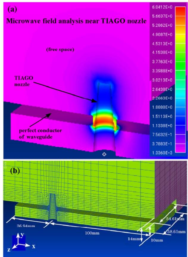
Fig.7 Numerical analysis on the spatial distribution of microwave electric field around the TIAGO nozzle by using PHOTO-Wavejω(Photon Co. Ltd.). (a) The distribution of microwave electric field, and (b) mesh structure for numerical analysis.
