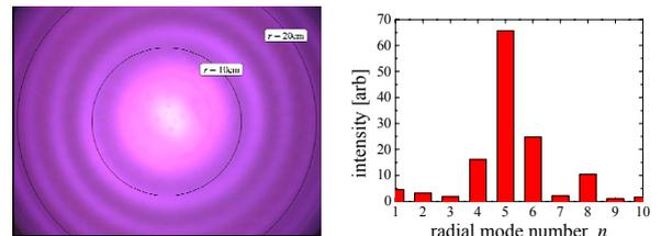
Fig. 4. (a) The light emission intensities measured by the CCD camera,  $P_{in} = 1.51$  kW,  $p = 200$  mTorr, and (b) the spectrum of the mode in the radial direction.
