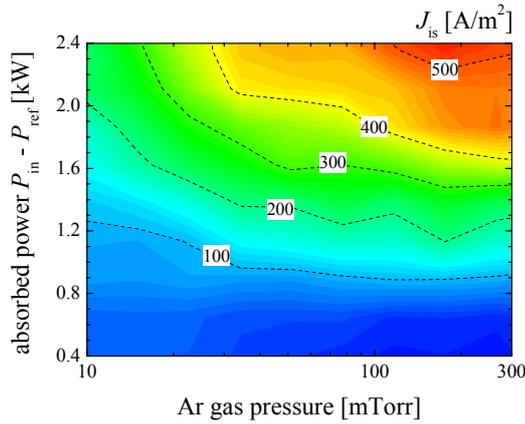
Fig. 2. The relationship of the ion saturation current density to the incident power and Ar gas pressure.
