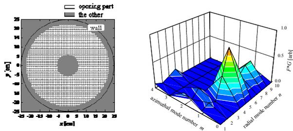
Fig. 7. (a) The aperture function, and (b) the radiated spectrum with the multi-slots antenna.
