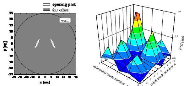
Fig. 8. (a) The aperture function, and (b) the radiated spectrum with a few slots antenna.
