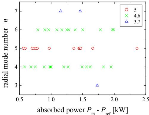
Fig. 6. The radial mode number  $n$  measured by the electric field probe.
