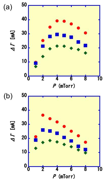
Fig.5 Pressure dependence of negative ion densities in the vicinity of the extraction electrode (i.e. the PG): (a) D<sub>2</sub> plasma and (b) H<sub>2</sub> plasma. Parameter is  $B_{MF}$ , i.e.  $B_{MF} = 80$  Gauss (●), 120 Gauss (■), 150 Gauss (◆). Experimental conditions are as follows:  $V_d = 70$  V,  $I_d = 10$  A and measurement point of  $\Delta I$   $z = -1.5$  cm.
