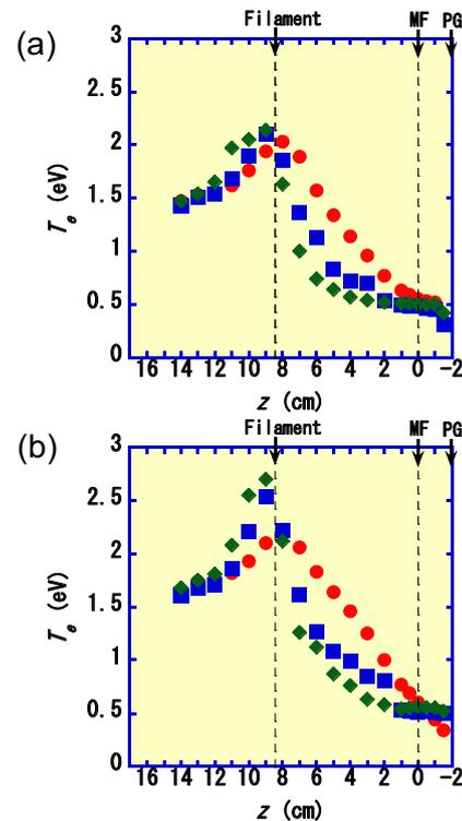
Fig.3 Axial distributions of electron temperature  $T_e$  in (a) D<sub>2</sub> and (b) H<sub>2</sub> plasmas. Parameter is the magnetic field intensity  $B_{MF}$  of the MF, namely  $B_{MF} = 80$  Gauss (●), 120 Gauss (■) and 150 Gauss (◆). Experimental conditions are as follows: discharge voltage  $V_d = 70$  V, discharge current  $I_d = 10$  A, gas pressure  $p$  (H<sub>2</sub>) = 2 mTorr and  $p$  (D<sub>2</sub>) = 4 mTorr
