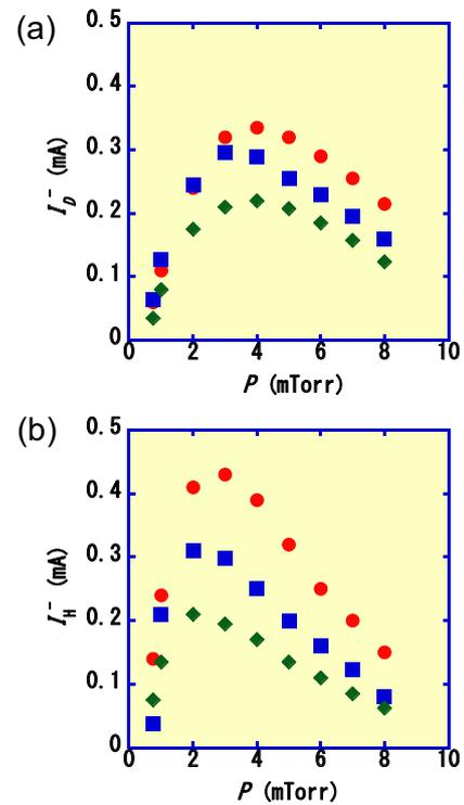
Fig.7 Pressure dependence of extracted D<sup>-</sup> current in (a) and H<sup>-</sup> current in (b), corresponding to the negative ion densities shown in Fig.5. Experimental conditions are the same as in Fig.5, where extraction voltage  $V_{ex} = 1.5$  kV.
