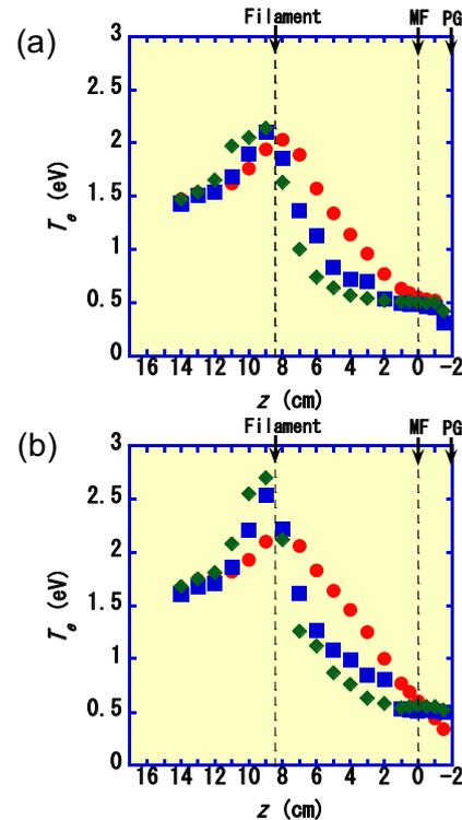
Fig.3 Axial distributions of electron temperature  $T_e$  in (a) D<sub>2</sub> and (b) H<sub>2</sub> plasmas. Parameter is the magnetic field intensity  $B_{MF}$  of the MF, namely  $B_{MF}$  = 80 Gauss (●), 120 Gauss (■) and 150 Gauss (◆). Experimental conditions are as follows: discharge voltage  $V_d$  = 70 V, discharge current  $I_d$  = 10A, gas pressure  $p$  (H<sub>2</sub>) = 2 mTorr and  $p$  (D<sub>2</sub>) = 4 mTorr
