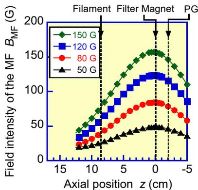
Fig.2 Axial distributions of field intensities for four different magnetic filters (MF),  $B_{MF}$
