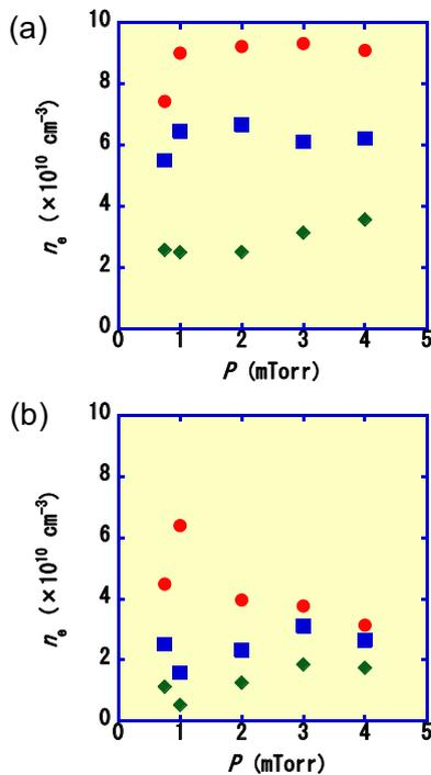
Fig.6 Pressure dependence of electron density in the vicinity of the PG: (a) D<sub>2</sub> plasma and (b) H<sub>2</sub> plasma. Parameter is  $B_{MF}$ , i.e.  $B_{MF} = 80$  Gauss (●), 120 Gauss (■) and 150 Gauss (◆). Experimental conditions are as follows:  $V_d = 70$  V,  $I_d = 10$  A and  $z = -1.5$  cm.
