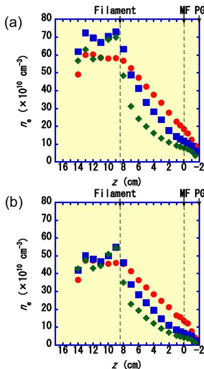
Fig.4 Axial distributions of electron density  $n_e$  in (a) D<sub>2</sub> and (b) H<sub>2</sub> plasmas. Parameter  $B_{MF}$  and experimental conditions are the same as in Fig.3.
