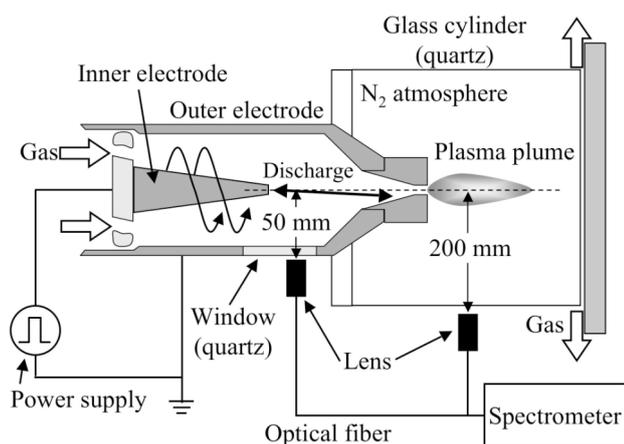
Fig. 1. A schematic view of the atmospheric plasma jet and the experimental set up.
