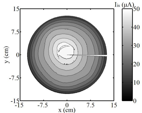
Fig. 6  $x$ - $y$  profiles of the ion saturation current  $I_{is}$  of the LP at  $z = 10$  cm in the diffusion chamber.
