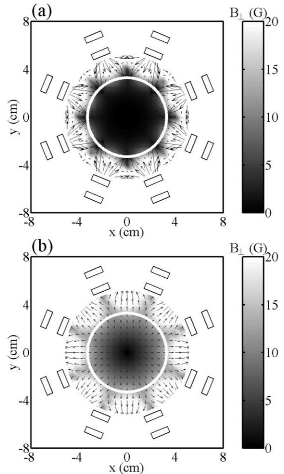
Fig. 3 The calculated  $x$ - $y$  profiles of the magnetic-field strength  $B_{\perp}$  in the direction perpendicular to  $z$ -axis at (a)  $z = -7$  cm and (b)  $z = -5$  cm in the source tube (contour plot), where the white circles and open rectangles show the glass wall and PMs having radially inward magnetization, respectively. The solid arrows indicate the local magnetic-field vector in the perpendicular direction.
