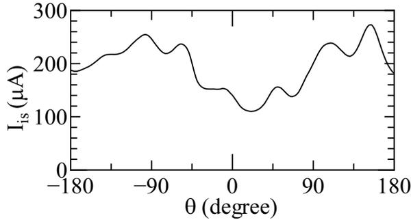
Fig. 4 Azimuthal profile of the ion saturation current  $I_{is}$  of the LP at  $z = -7$  cm and  $r = 2.6$  cm in the source tube, where the LP is biased at  $-60$  V to collect ions and  $\theta = 0$  is defined as the left side in Fig. 5-6.
