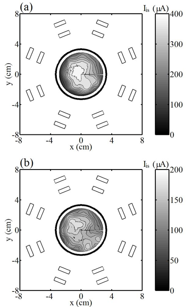
Fig. 5  $x$ - $y$  profiles of the ion saturation current  $I_{is}$  of the LP at (a)  $z = -7$  cm and (b)  $z = -5$  cm in the source tube, where the bold lines and open rectangles show the glass wall and PMs having radially inward magnetization, respectively.
