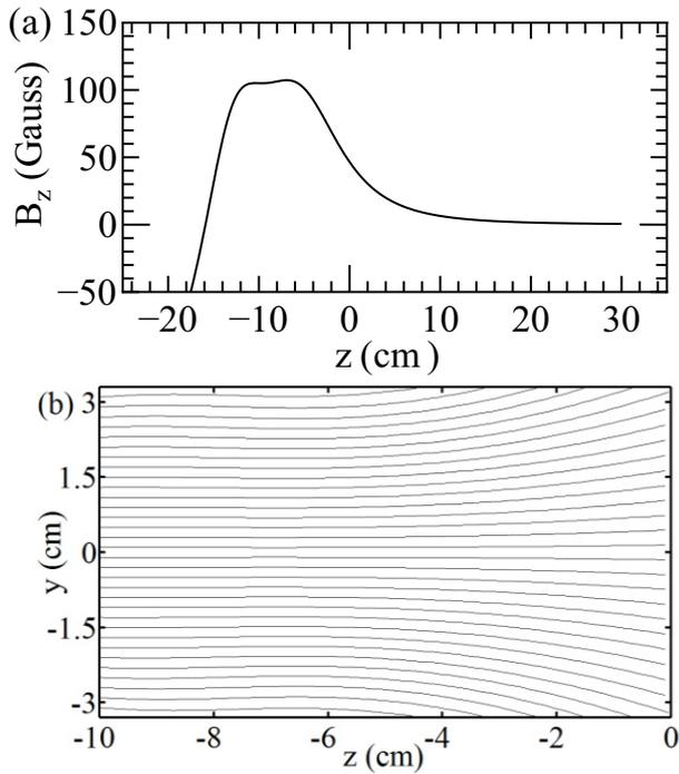
Fig. 2 (a) Axial profile of the calculated axial component  $B_z$  of the magnetic-field strength produced by the PMs arrays presented at the left of Fig. 1. (b)  $z$ - $y$  profile of the field-line structures in the source tube.
