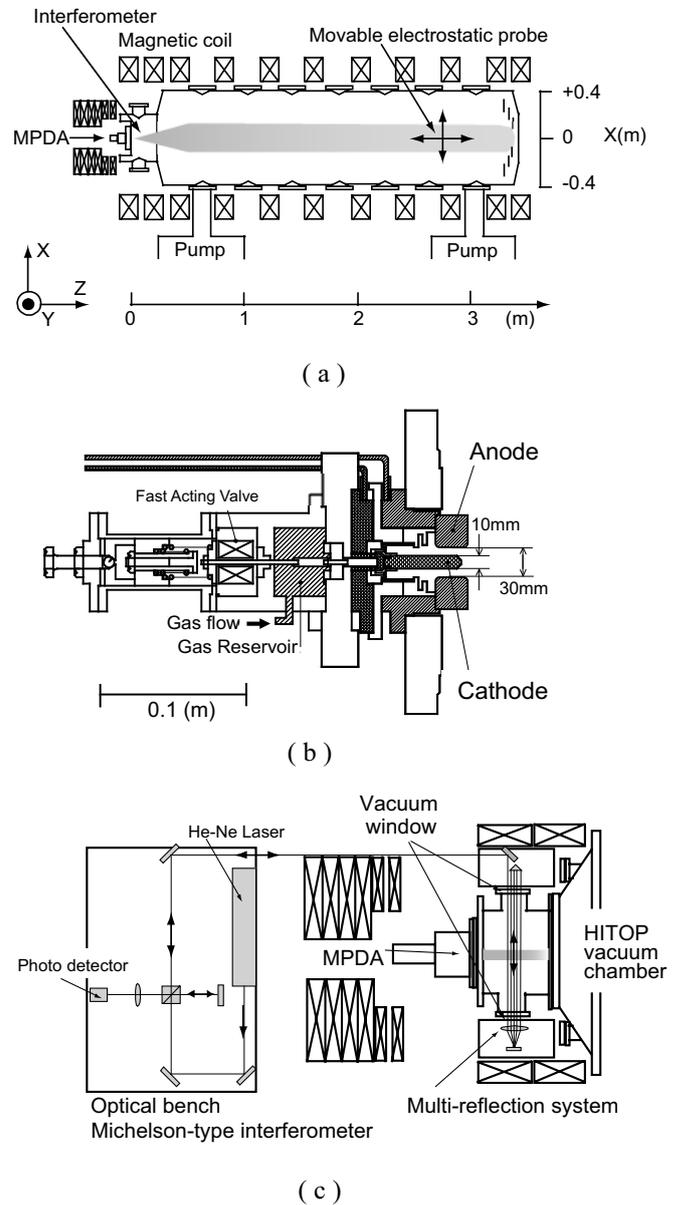
Fig. 2 Schematic views of (a) the HITOP device, (b) the MPDA device and (c) the multi-reflection type laser interferometer.
