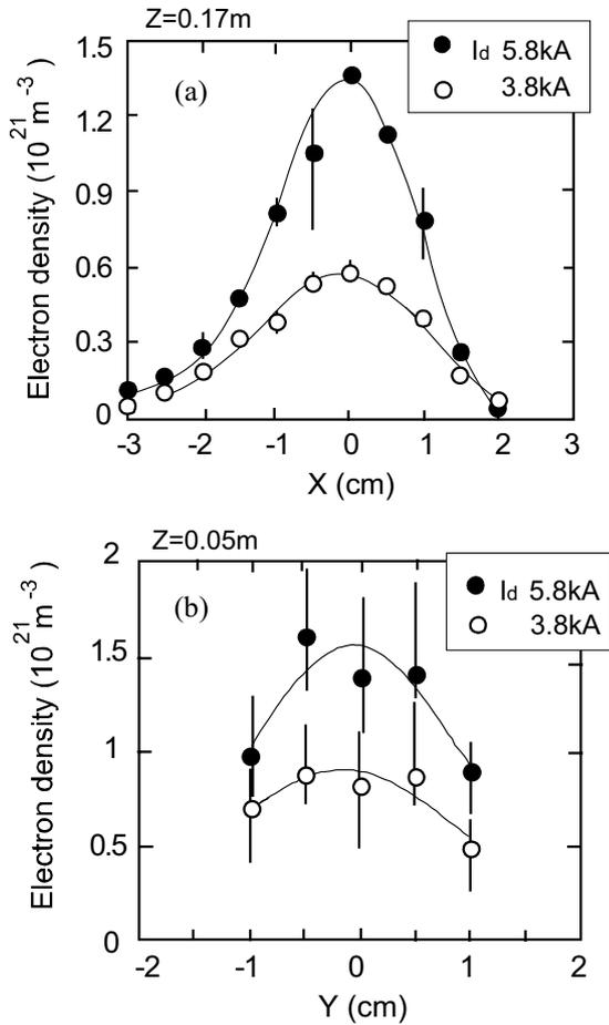
Fig. 3 Electron density profiles measured by the electrostatic probe(a) and the interferometer(b).
