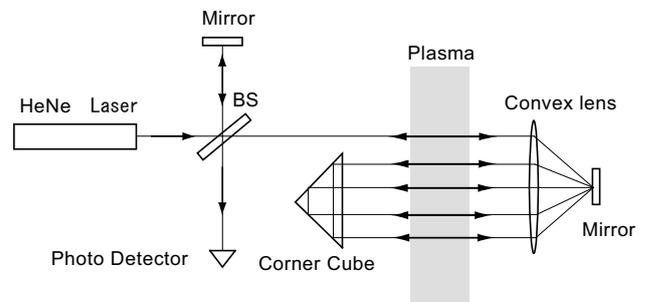
Fig.1. Schematic view of the multi-reflection type laser interferometer
