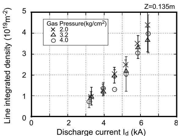
Fig.4 Dependence of the line integrated density with the discharge current  $I_d$ .
