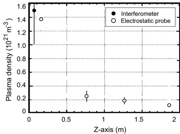
Fig. 5 Axial profile of the plasma density measured by the interferometer and the electrostatic probes. (Discharge current  $I_d=5.4\text{kA}$ , Uniform magnetic field strength= $0.087\text{T}$ ).
