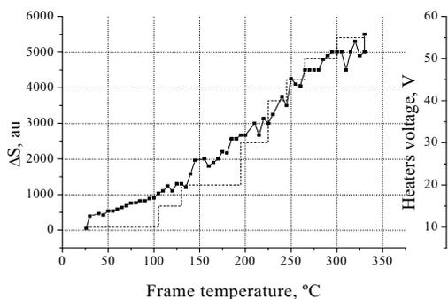
Fig.2 sensitivity over frame temperature
