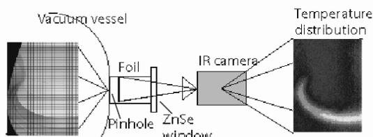
Fig.1 imaging bolometer layout
