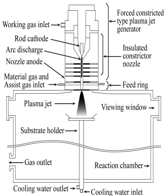
Fig.1. Schematic diagram of thermal plasma reactor with plasma jet system.
