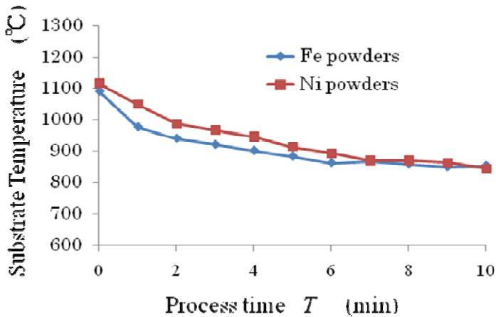
Fig.3. Substrate temperature by an increase of time, corresponding to Fig 2
