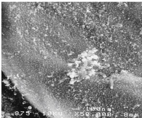
Fig.3 FE-SEM image of the surface of a sample stainless steel 304 substrate after the CNT formation PCVD process. A few fibers can be seen near the center of the image.
