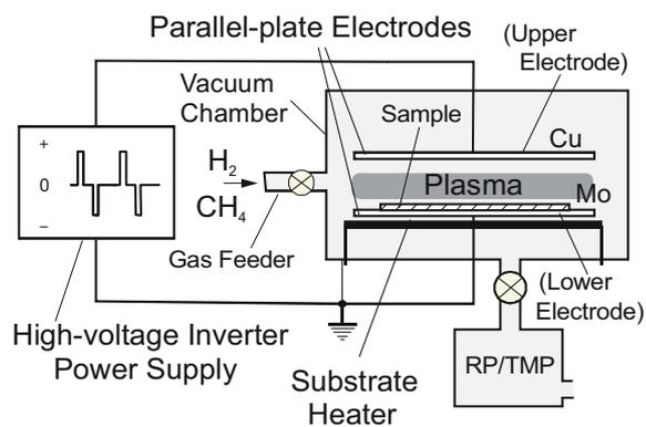
Fig.1 Schematic diagram of the PCVD apparatus for CNT formation. This system has been developed by ULVAC, Inc. and Osaka Univ.
