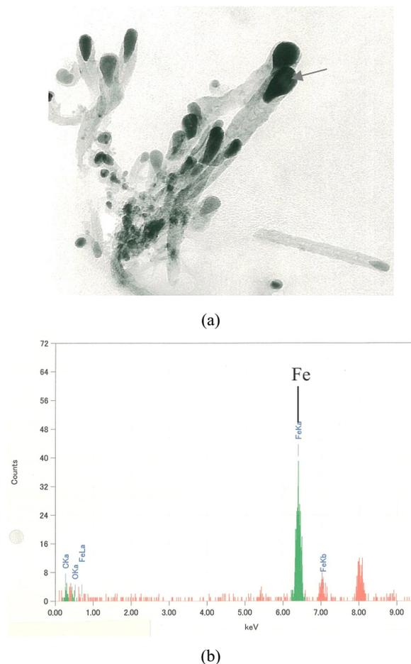
Fig.5 Results of TEM-EDX analysis of the particles included in CNTs
