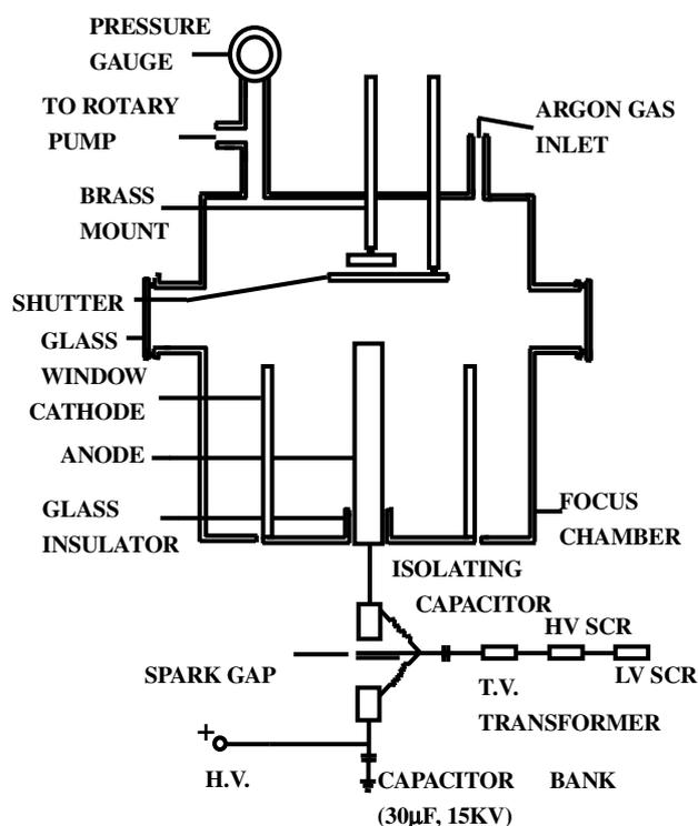
Fig.1. Dense Plasma Focus device with its modifications
