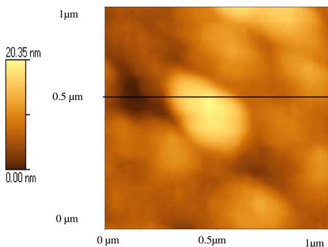
Fig.5. AFM image of zinc oxide nanoparticles
