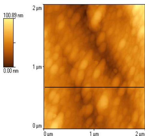
Fig.6. AFM image of cobalt nanoparticles
