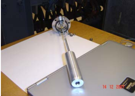
Fig.6 In-vacuum fiber probe for spectroscopic measurements.
