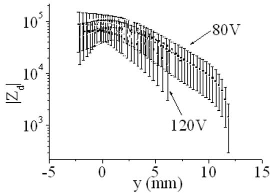
Fig. 6 Charge number  $|Z_d| = |Q|/e$  as a function of the vertical position  $y$  with 80V and 120V applied between parallel electrodes.
