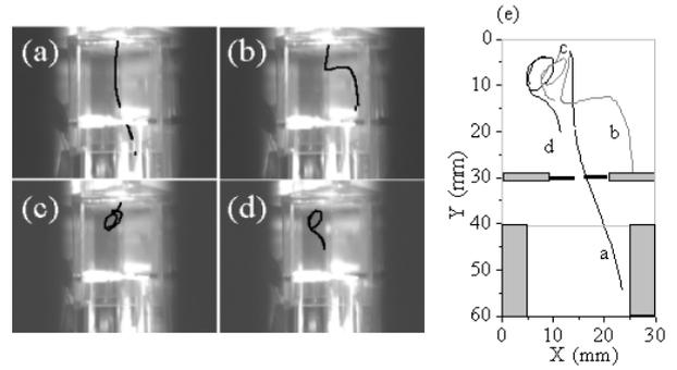
Fig. 4 (a)-(d): Photographs with particle trajectories in liquid helium vapor when 200V is applied to left-hand side of parallel electrodes while right-hand side electrode is grounded (Electric field  $E\sim 7$ kV/m). The radius of particles is  $1.5\mu\text{m}$ . (e): The trajectories were plotted with apparatus configuration of transparent rectangular parallelepiped acrylic tube.
