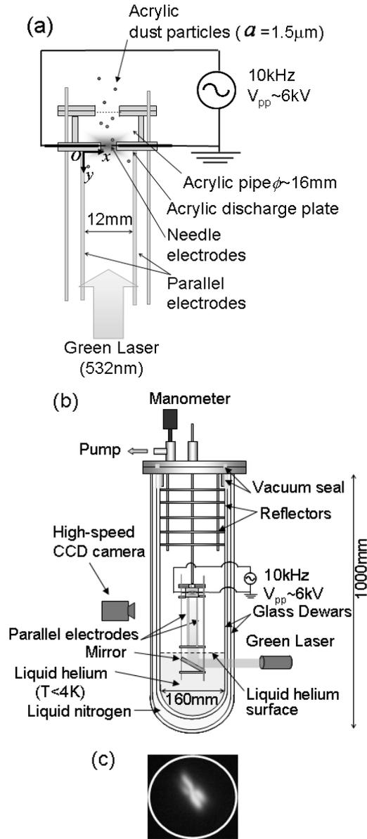
Fig. 1 (a) Schematic diagram of the measurement system. (b) Cryogenic glass Dewar system to impound liquid helium with temperature less than 4K. Green laser and camera are set in front of 20mm-wide optical slits. (c) Snapshot of plasma in liquid helium vapor.
