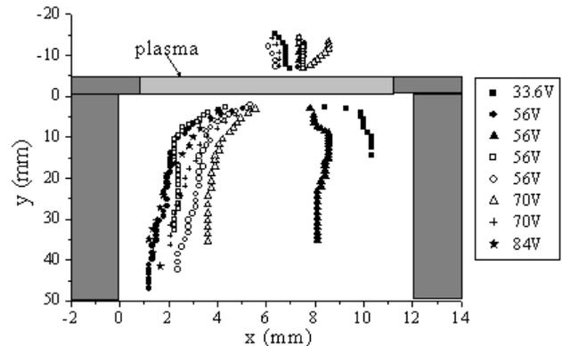
Fig. 2 Dust particle trajectories in liquid helium vapor, when 30~90V was applied between the parallel electrodes (The right-hand side electrode was grounded). The radius of particles is 1.5 $\mu\text{m}$ . Liquid helium surface is at  $y \sim -100$ mm.
