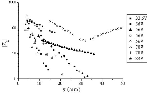
Fig. 3 Estimated dust charge from trajectories plotted with closed squares in Fig. 2 as a function of vertical position  $y$ .
