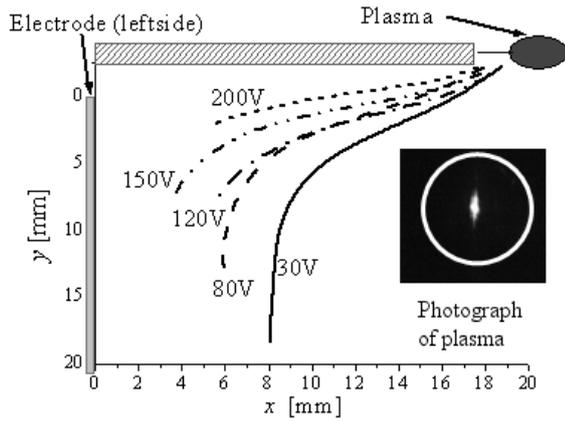
Fig. 5 Typical trajectories of dust particles with radius of  $5\mu\text{m}$  in atmospheric-pressure helium plasma at 300K. The number labeled to each trajectory represent the applied voltage to the left-hand side electrode while right-hand side electrode is grounded.
