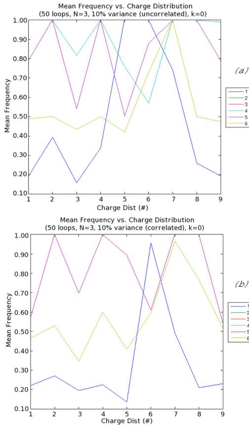
Fig. 3 Dependence of the mean frequencies of the normal modes for different charge distributions in the case of uncorrelated, (a), and correlated, (b) fluctuations.
