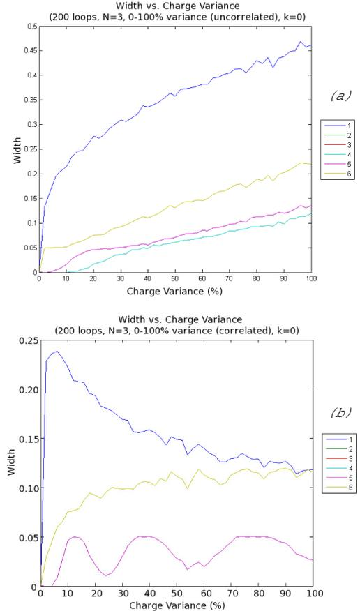
Fig. 2 Dependence of the half-width of the normal modes on the charge variance in the case of uncorrelated, (a), and correlated, (b) fluctuations.
