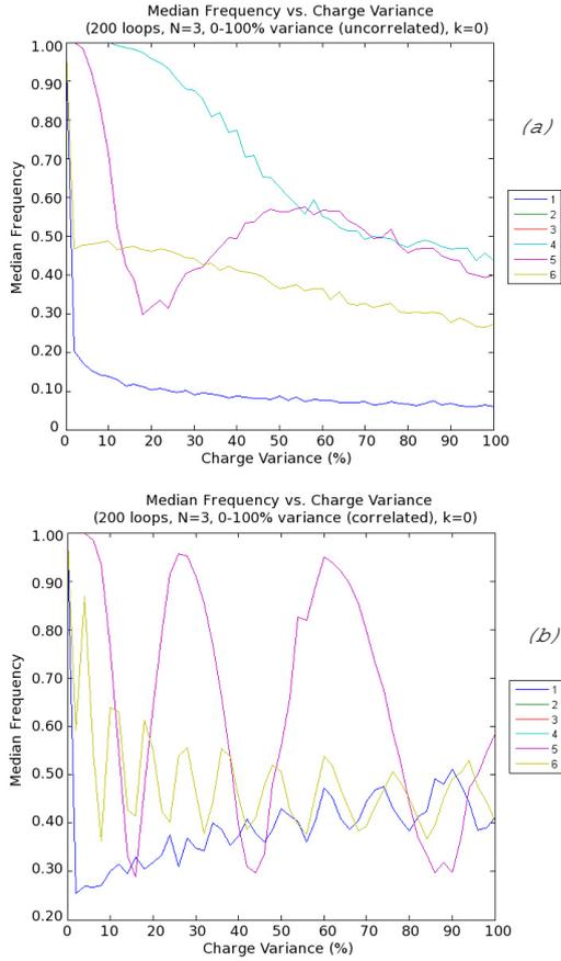
Fig. 1 Dependence of the mean frequency of the normal modes (see legend on the figure) on the charge variance in the case of uncorrelated, (a), and correlated, (b) fluctuations.
