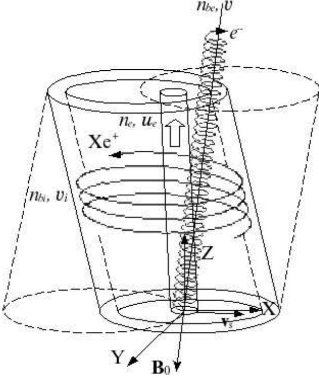
Fig. 1 Electron beam injection ( $e^-$ ) directed through the hollow beam of xenon ions ( $Xe^+$ ) with the beam density and velocity  $n_{be}, v$  and  $n_{bi}, v_i$ , respectively. Release of the electron flow with the density and stream velocity  $n_e, u_e$  for a compensation of the ion beam charge at the output of SPT is shown by the uparrow. Here,  $B_0$  and  $v_s$  are the directions of the quasi-steady magnetic field and the satellite velocity in the  $X, Y, Z$  coordinate system.
