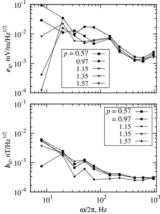
Fig. 4 Spectra of the electric and magnetic component of ELF-ULF waves,  $e_{lf}$ ,  $b_{lf}$ , respectively, are measured at *IK-25* in the frequency range 8-969 Hz for different parameter values  $p$  (see Fig. 3.).
