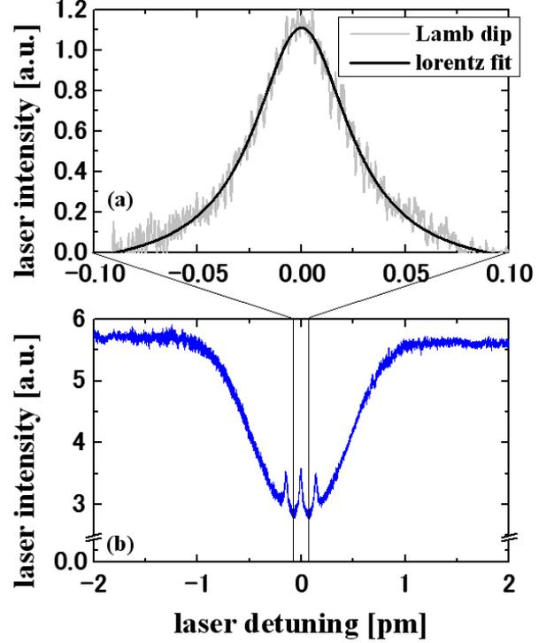
Fig. 4 Lamb dip component (a) and the saturated absorption spectrum (b).
