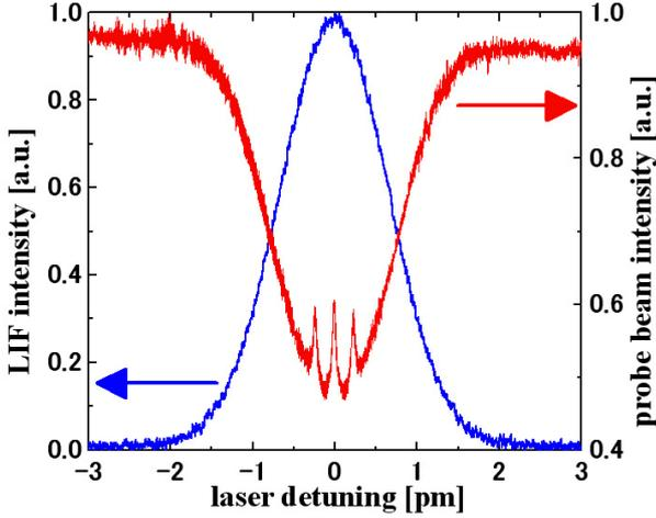
Fig. 3 LIF and saturated absorption spectra. There are three Lamb dips at the resonant wavelength (bottom of the absorption spectrum).
