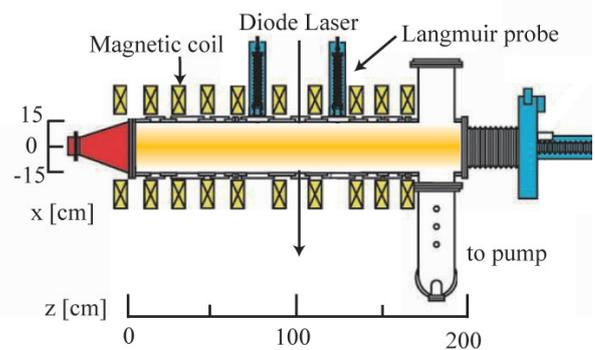
Fig. 1 Schematic of HYPER-I device.
