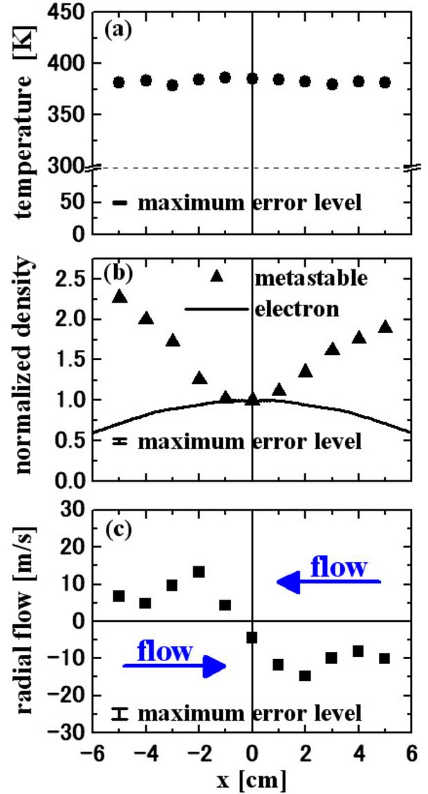
Fig. 7 Metastable temperature, density, radial flow and electron density profile. The flow direction of metastable (neutral) particles is inward. The metastable and electron density are normalized at  $x = 0$ , respectively. The electron density at  $x = 0$  is about  $4.8 \times 10^{10} \text{cm}^{-3}$
