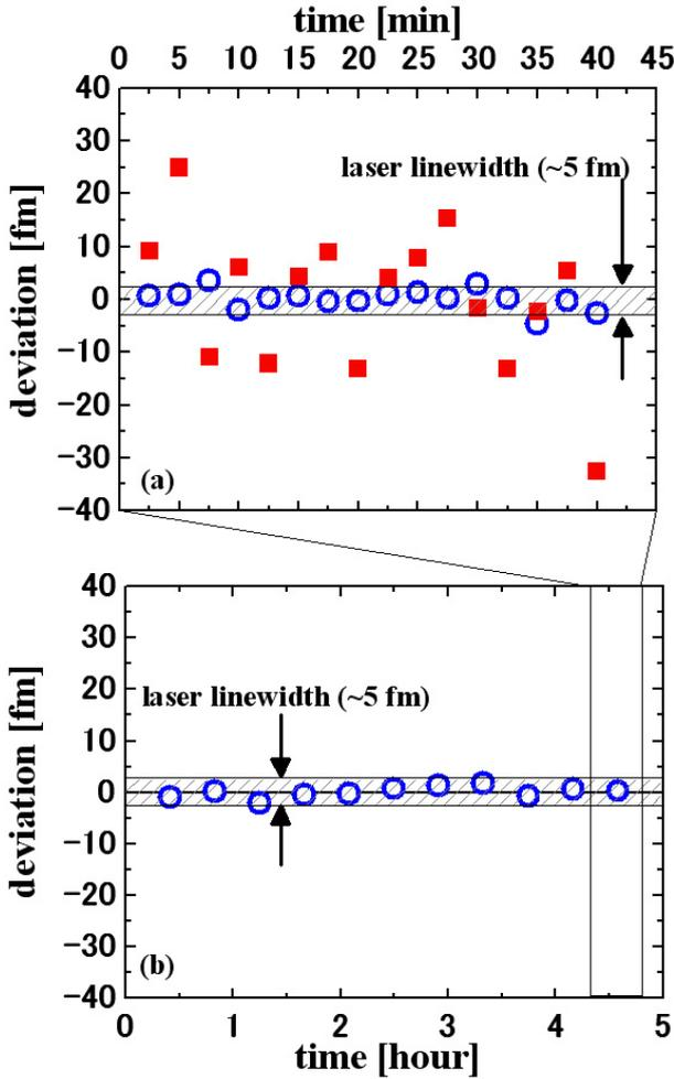
Fig. 6 Deviation of LIF peak position in wavelength for the repeated measurements under the same experimental condition. (a): short term; (b): long term. The reference of laser wavelength is Lamb dip (open circles) or iodine absorption spectrum (closed square).
