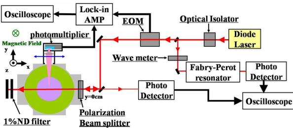
Fig. 2 LIF spectroscopy system.
