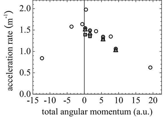
Fig. 6  $L$  dependence of the acceleration rate. The closed and open symbols mean the experimental conditions at 0.1 [mTorr] and 0.2-0.4 [mTorr], respectively.
