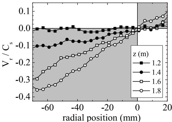
Fig. 5 Radial profiles of radial flow velocity at different axial positions.
