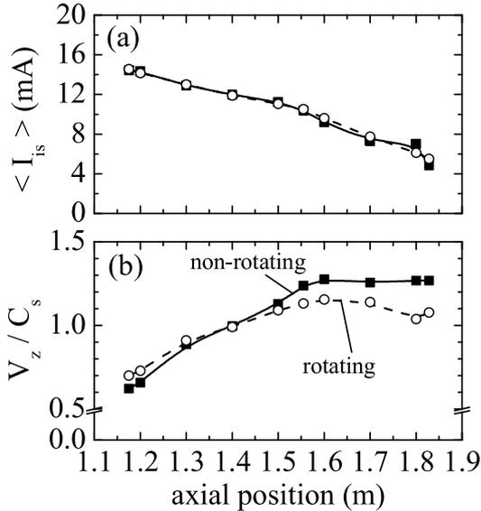
Fig. 3 Axial profiles of the density (a) and the axial flow velocity (b). The square with solid lines is for a rotating plasma case, and the open circle with dashed line is for a non-rotating plasma case.
