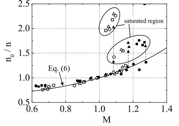
Fig. 4 Density ratio as a function of Mach number. The closed and open symbols mean the non-rotating plasma case and the rotating plasma case, respectively. The data at  $r = 0, 30$  and  $50$  [mm] are presented by squared boxes, circles and triangles, respectively.
