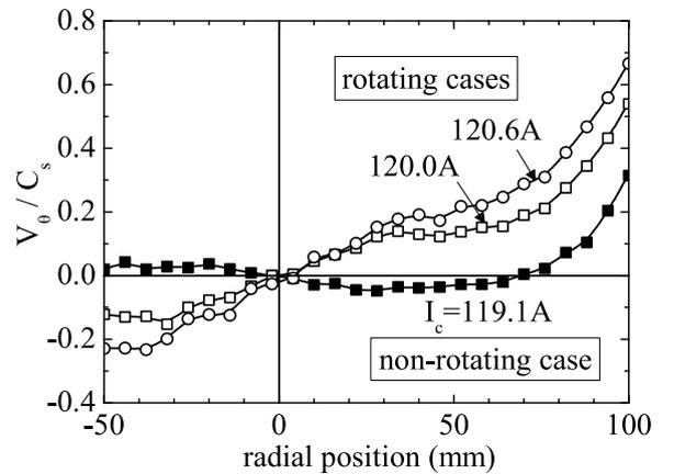
Fig. 2 Radial profiles of azimuthal ion flow velocity. Rotating plasma cases (open symbols) and non-rotating plasma case (closed symbol).
