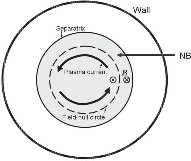
Fig. 1 Two dimensional geometry of tangential neutral beam injection. The beam trajectory is shifted from the center, and it is almost tangential to the field-null circle.
