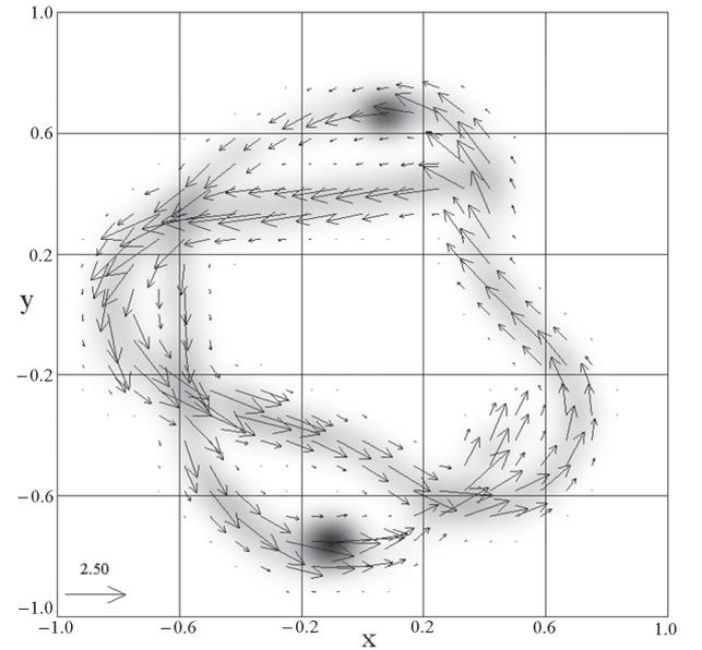
Fig. 2 Flow velocity profile of neutral beam injected fast hydrogen ions. Here,  $x$  and  $y$  are normalized by the wall radius. The beam flow velocity is normalized by the plasma ion thermal velocity  $\sqrt{2T_i/m_i}$ . The reference arrow is drawn in the left bottom corner, and its length corresponds to  $2.5 \sqrt{2T_i/m_i}$ .
