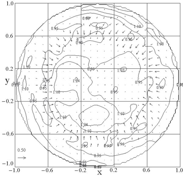
Fig. 3 Contour of electron density and electric field profile at  $t=10/\omega_{ci0}$  where  $\omega_{ci0} \equiv qB_{ex}/m_i$ . Electron density is normalized by  $5.0 \times 10^{19} \text{ m}^{-3}$ . The values on the contour line represent value of the normalized density. The reference arrow is drawn in the left bottom corner, and its length corresponds to  $0.5 B_{ex} \sqrt{2T_i/m_i}$ .
