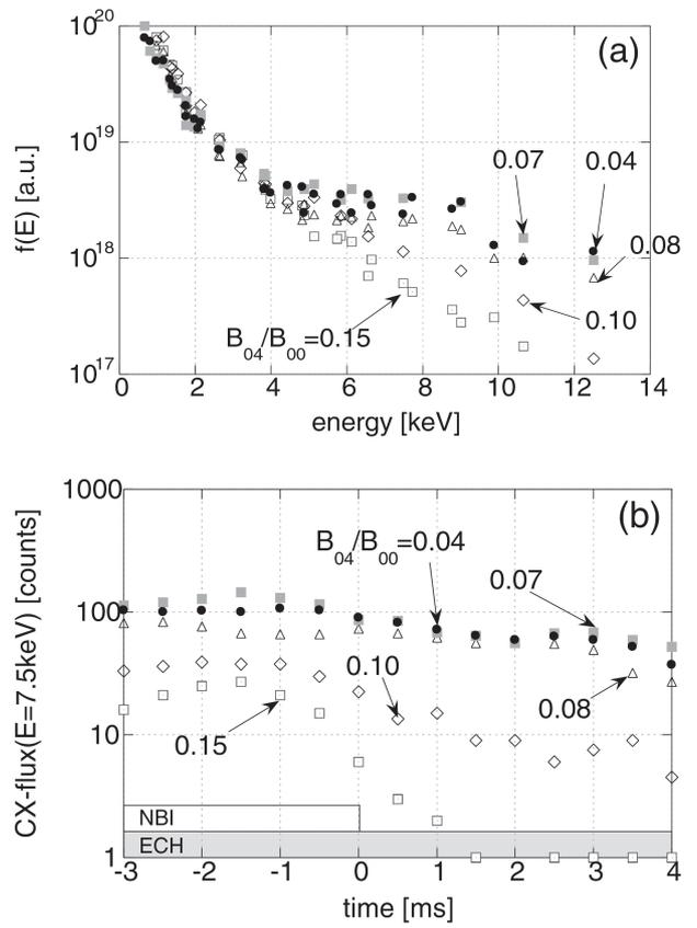
Fig. 4 (a) energy spectra during NBI and (b) the time evolution of CX-flux with energy of 7.5 keV measured in the bumpiness control experiment.
