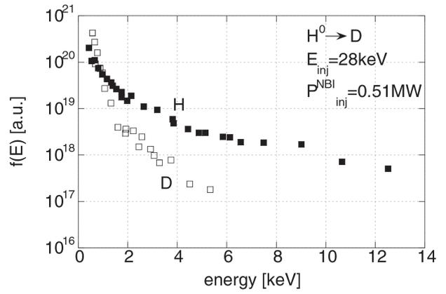
Fig. 2 Energy spectra measured with CX-NPA in NB injection into deuterium plasma.
