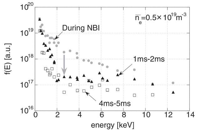
Fig. 3 The energy spectra at 1–2 ms, 4–5 ms after termination of NBI. The energy spectra during NBI are also shown.
