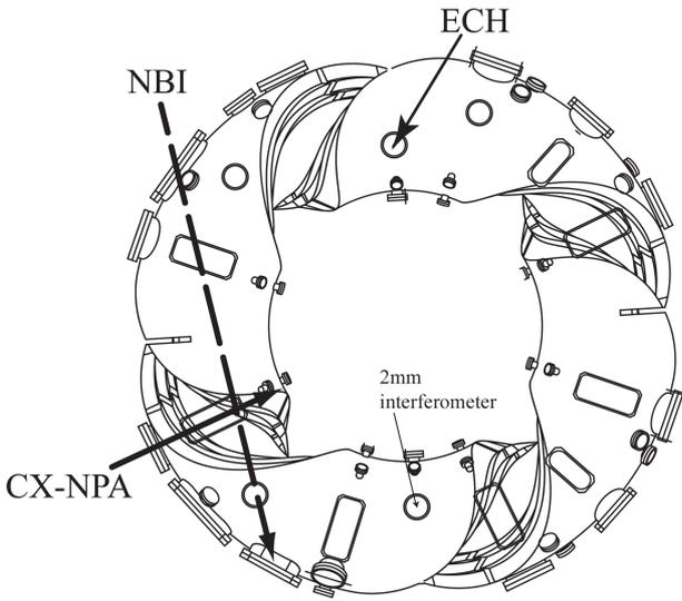
Fig. 1 Experimental set-up of NBI and CX-NPA systems.
