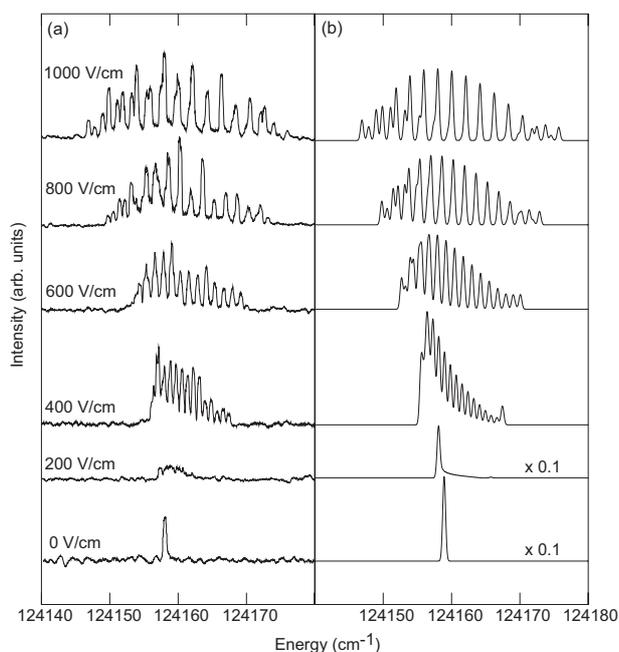
Fig. 3 Comparison between (a) experimental and (b) calculated Stark spectra of the  $N^+ = 2$ ,  $n = 16$ ,  $M_J = 0$  Stark manifold. The simulation has been convoluted with a Gaussian laser bandwidth with full width at half maximum of  $0.5 \text{ cm}^{-1}$ .
