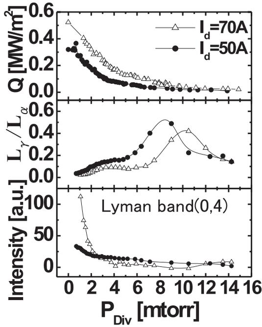
Fig. 2 The effect of hydrogen neutral gas pressure,  $P_{Div}$ , on the heat to the target plate,  $Q$ , the hydrogen Lyman spectrum ratio,  $L_\gamma/L_\alpha$ , and the intensity of VUV emission spectrum at the Lyman-band system ( $B^1\Sigma_u^+ \rightarrow X^1\Sigma_g^+$ ) at various discharge current  $I_d$ . The  $I_d$  changes (●) 50, and (△) 70 A.
