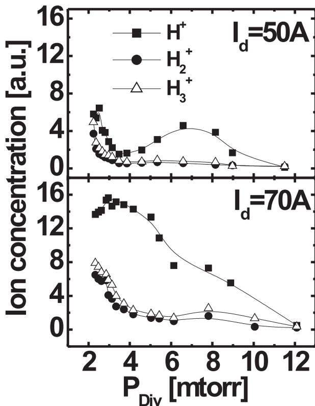
Fig. 4 The relative ion concentrations as function of  $P_{Div}$  at the discharge current  $I_d$  of 50 and 70 A at the magnetic field  $B$  of 0.78 kG.
