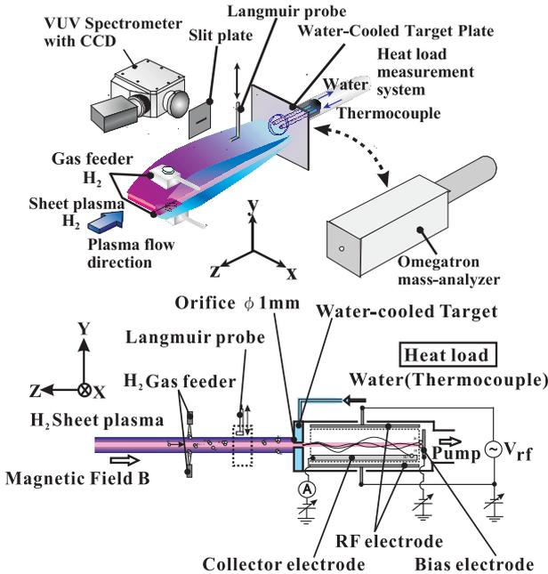
Fig. 1 Schematic diagram of the magnetized plasma simulator (sheet plasma device) TPD-SheetIV and detection system.
