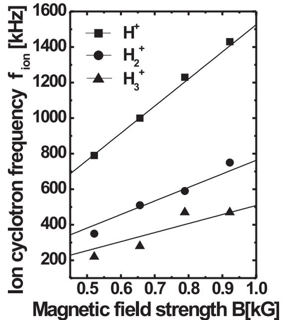
Fig. 3 The measured resonance frequency  $f_{ion}$  as function of the magnetic field strength  $B$  at the discharge current  $I_d$  of 50 A and the  $P_{Div}$  of 4 mtorr. The value of  $B$  changes from 0.5 to 1.0 kG. From the typical plasma omegatron experiment, it can be seen that the peaks correspond to  $H^+$ ,  $H_2^+$ ,  $H_3^+$ .
