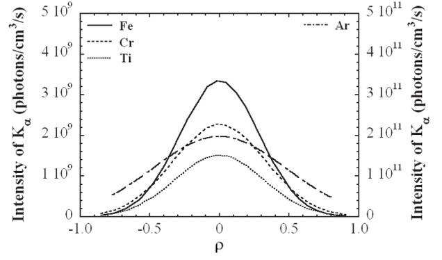
Fig. 5 Typical radial emissivity of  $K_{\alpha}$  line emitted from argon (chain line) and heavy metallic impurities such as titanium (dotted line), chromium (broken line), and iron (solid line).  $K_{\alpha}$  profiles were fitted by Gaussian.
