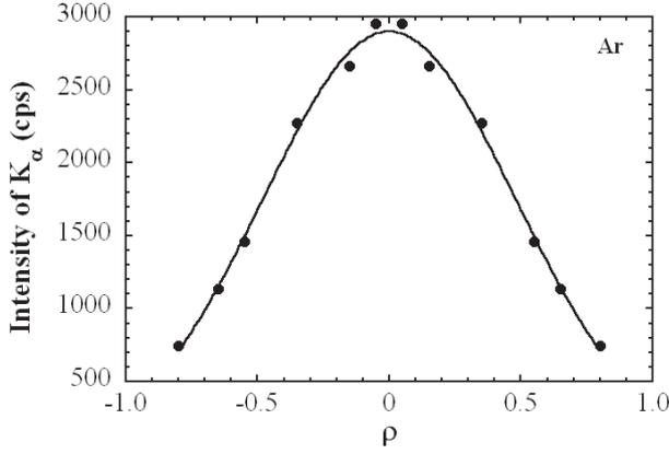
Fig. 4 Typical radial profiles of Ar  $K_{\alpha}$  lines. Solid line indicates a Gaussian fitting. The data are obtained with an accumulation time of 50 msec.
