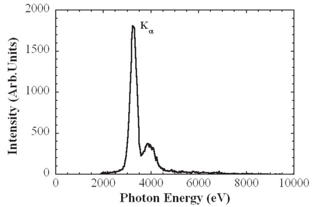
Fig. 2 Typical spectrum from Ar discharges in LHD.
