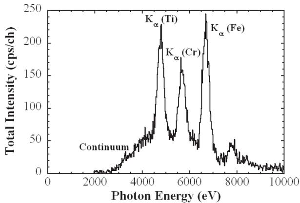
Fig. 1 Typical spectrum obtained from  $H_2$  and He discharges in LHD. Spectrum was measured with the PHA assembly. Lines denoted with  $K_\alpha$  (Ti),  $K_\alpha$  (Cr) and  $K_\alpha$  (Fe) indicate the  $K_\alpha$  lines of titanium, chromium, and iron, respectively.
