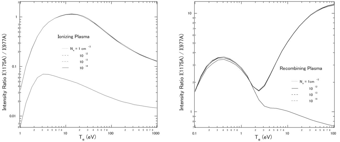
Fig. 1 Calculated intensity ratio of C<sup>2+</sup> lines in ionizing (a) and in recombining plasma (b).
