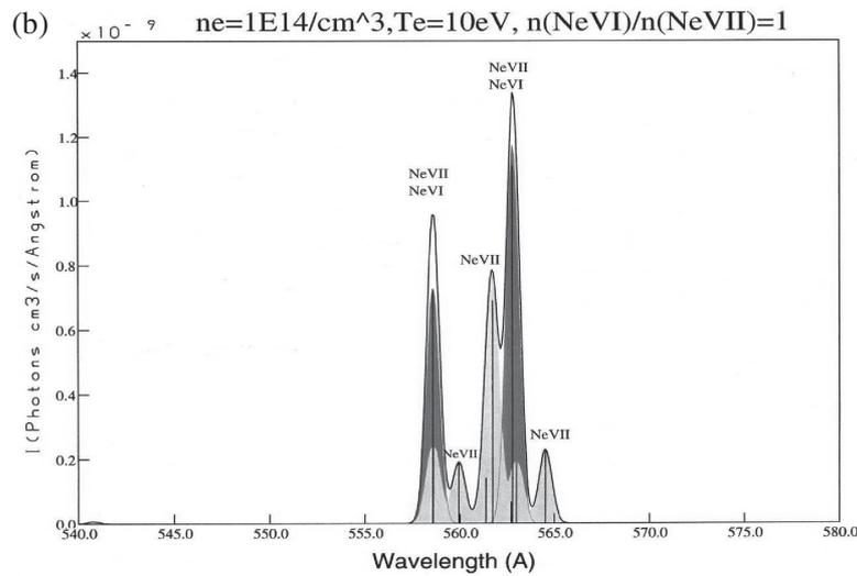
Fig. 4 Observed (a) and theoretical (b) spectra of NeVII and NeVI ions.
