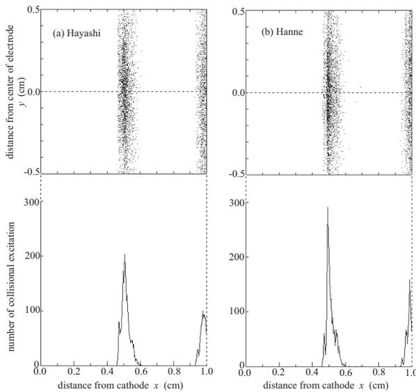
Fig. 3 Spatial distributions of excitation obtained by using cross sections shown in Fig. 2 ( $E/p_0 = 10 \text{ V/cm} \cdot \text{Torr}$ ,  $p_0 = 1 \text{ Torr}$ ).
