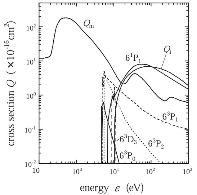
Fig. 1 Electron collision cross section of mercury. (to distinguish the cross sections, the line kind is indicated as for  $6^3P_1$  (broken line),  $6^3P_2$  (dotted line) and  $6^3D_3$  (long broken line).)
