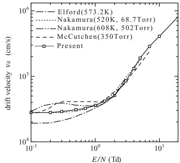
Fig. 4 Comparison between present result and experimental values of the drift velocity reported by other researchers.
