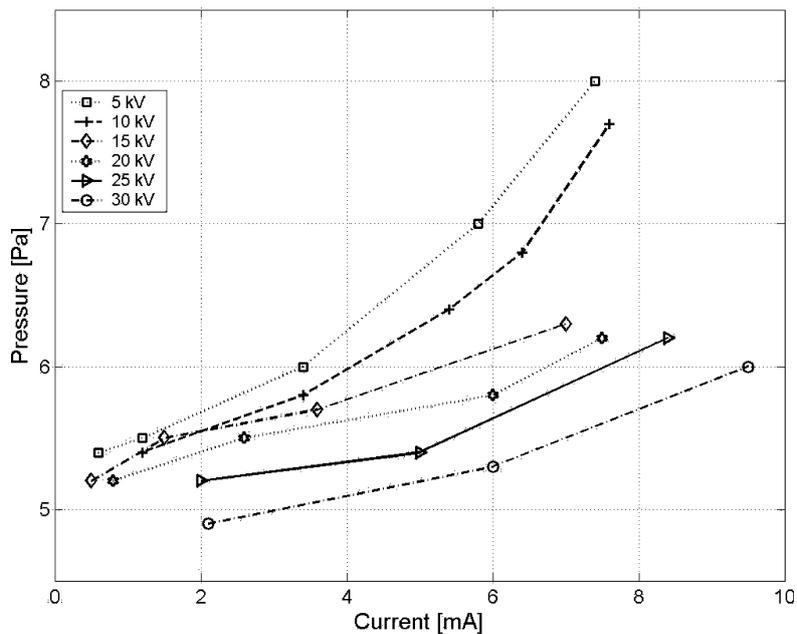
Fig. 3 Pressure vs. current measured at target plate for given voltages.
