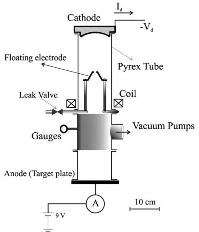
Fig. 1 Schematic structure of the electron gun with a concave cathode.
