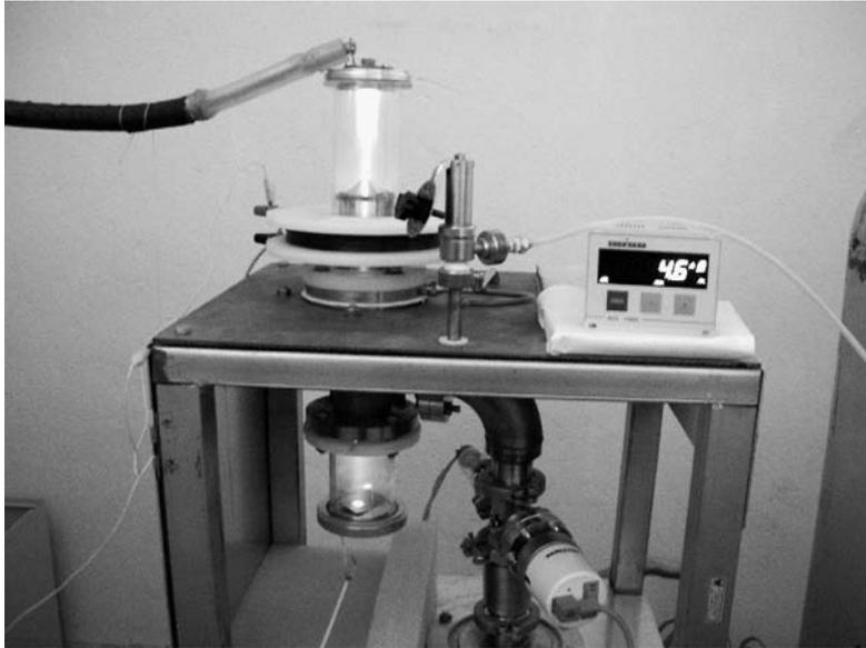
Fig. 2 Constructed electron gun facility in an experiment.
