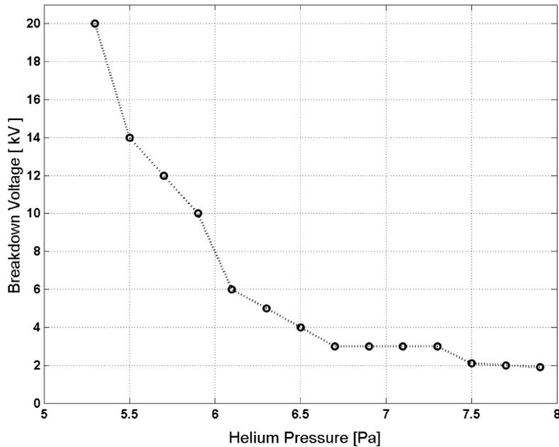
Fig. 4 Experimental breakdown curve.
