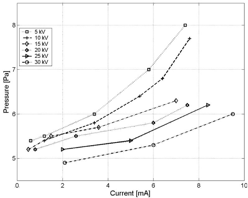
Fig. 3 Pressure vs. current measured at target plate for given voltages.
