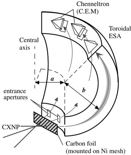
Fig. 4 The schematic view of a designed neutral particle analyzer.
