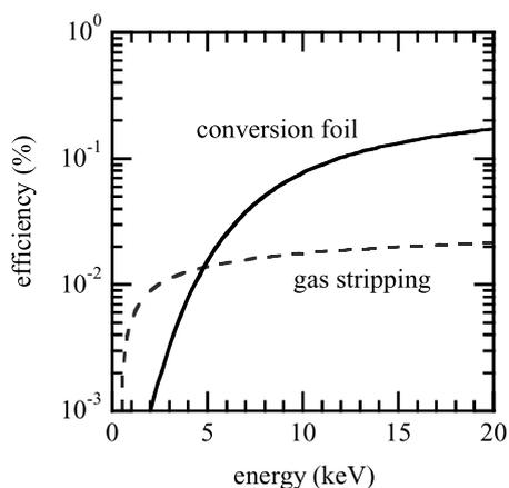
Fig. 6 Detection efficiency, including the conversion efficiency and the geometrical factor.
