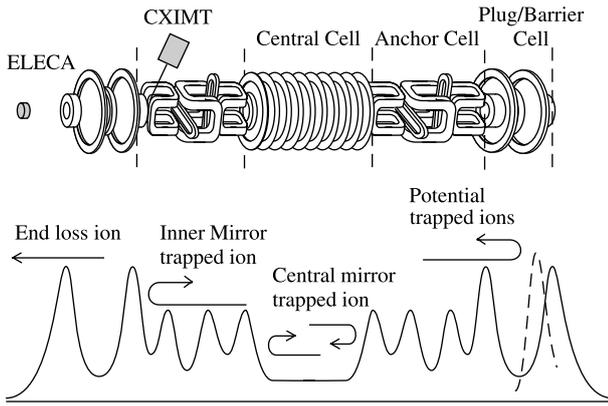
Fig. 1 The axial profile of magnetic field strength in the GAMMA 10, the kind of trapped ions and the location of CXIMT and ELECA. The confinement potential (dashed line) is generated in the plug/barrier cell.
