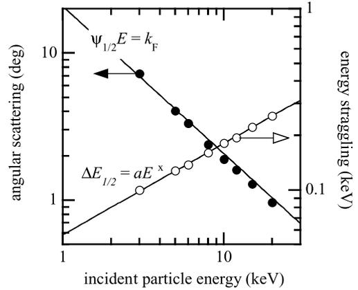
Fig. 5 HWHM of the angular scattering (closed circles) and the energy straggling (open circles) of transmitted particles.
