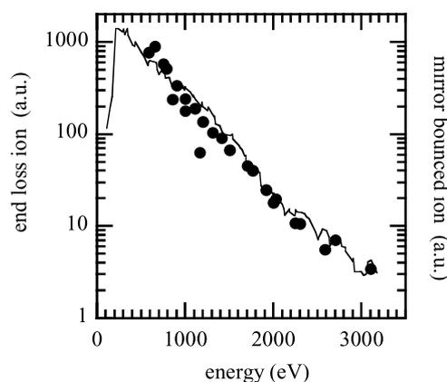
Fig. 3 Comparison of energy spectrum between end loss ions obtained by ELECA (solid line) and bounced ions taken by CXIMT.
