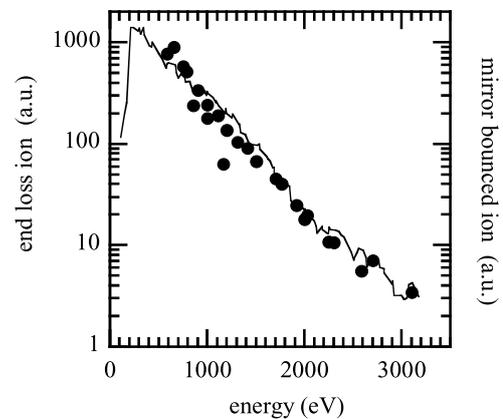
Fig. 3 Comparison of energy spectrum between end loss ions obtained by ELECA (solid line) and bounced ions taken by CXIMT.
