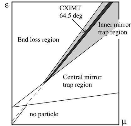
Fig. 2 Trap regions, end loss region and CXIMT measurement region in  $\epsilon$ - $\mu$  space, without the confinement potential.
