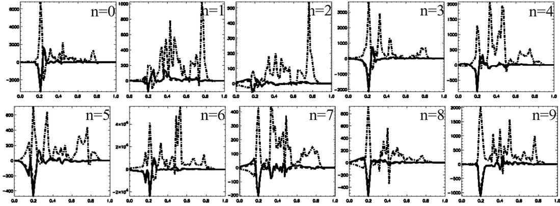
Fig. 1 Radial profile of absorbed power.  $n$  is toroidal mode number of wave electric field. Solid, broken, and broken-dotted lines are the power absorption by electron, helium, and hydrogen, respectively.
