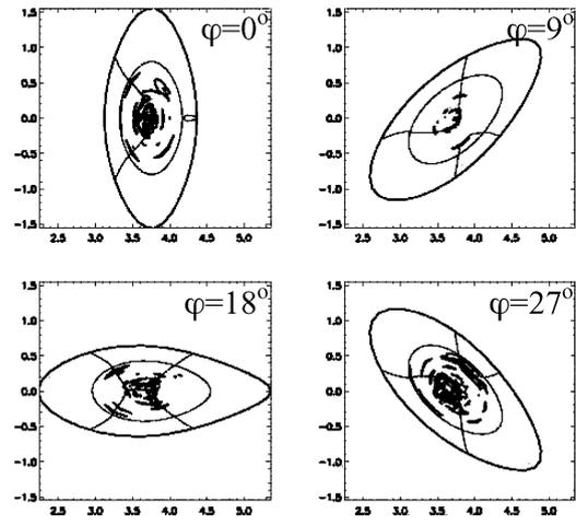
Fig. 5 Absorbed power in poloidal cross-section. Magnetic field is 2.61 T.
