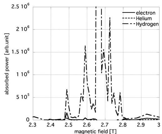
Fig. 2 Power absorption dependence on magnetic field. Solid, broken, and broken-dotted lines are the power absorption by electron, helium, and hydrogen, respectively.
