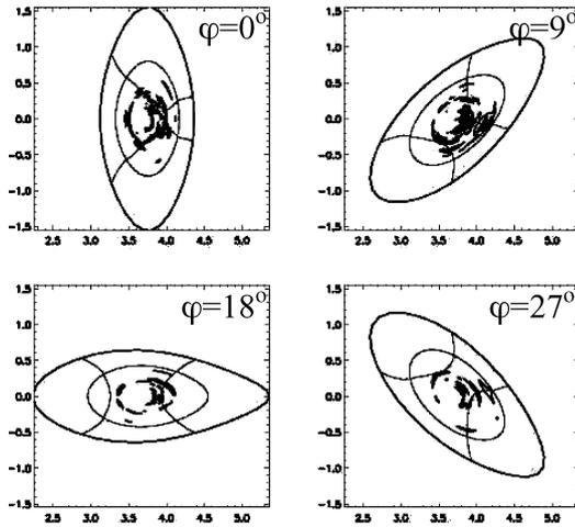
Fig. 3 Absorbed power in poloidal cross-section. Magnetic field is 2.75 T.  $\varphi$  is toroidal angle. Antenna is located at  $\varphi = 0^\circ$ . Ion cyclotron resonance layer, vacuum vessel and plasma surface are also plotted.
